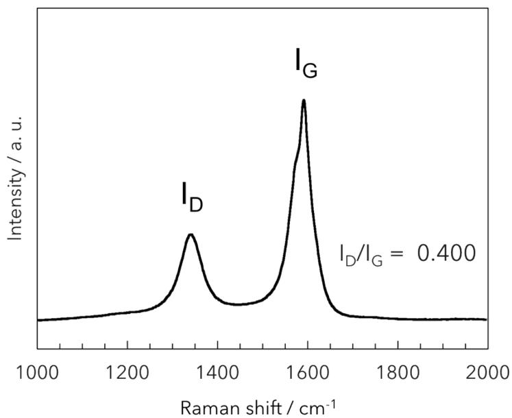
Fig. S1 Raman spectrum for the pristine super growth (single-walled) carbon nanotube (SGCNT) with the  $I_D/I_G = 0.40$ . The measurement was conducted on the bundled position of SGCNT by Raman spectroscopy systems (Horiba Jobin-Yvon, LabRam HR evolution).
