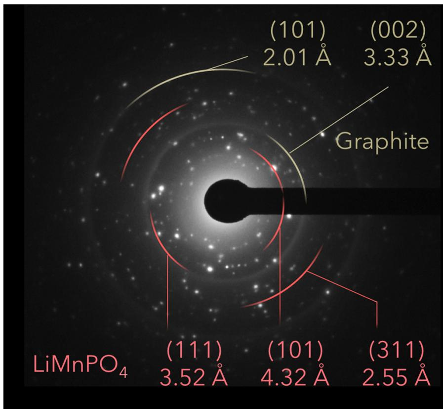
Fig. S4 Electron diffraction patterns for  $\text{LiMn}_{0.792}\text{Fe}_{0.198}\text{Mg}_{0.010}\text{PO}_4/\text{SGCNT}$  (their HRTEM images are shown in Fig. 2), indicating that those patterns are identical to  $\text{LiMnPO}_4$  and graphite attributed to the basal plane of SGCNT.
