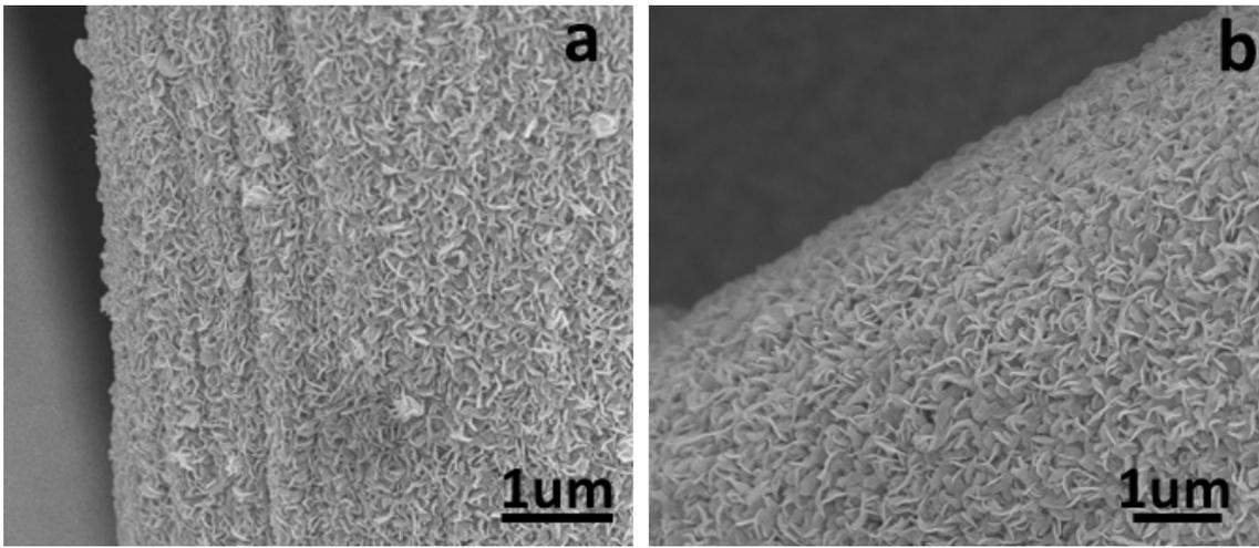
Figure S8. SEM image of MoS<sub>2</sub>/CC (a) and WS<sub>2</sub>/CC (b) after sonication for 30 min
