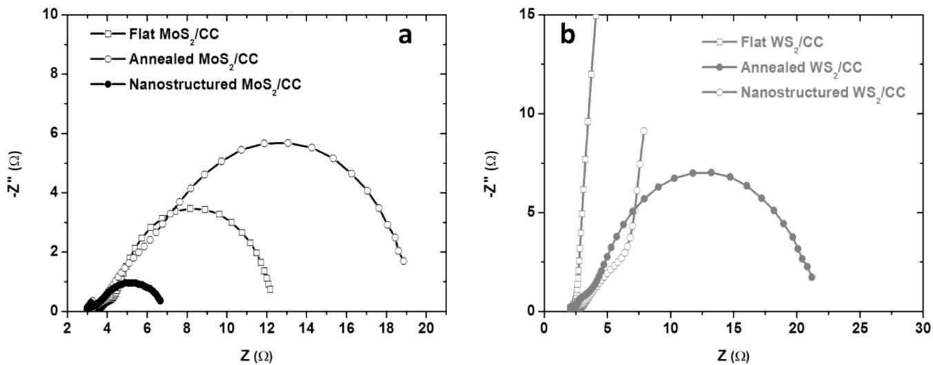
Figure S5. Nyquist plots of different samples. The electrochemical impedance spectroscopies (EIS) further reveal similar system resistance ( $R_s$ ,  $2.5 \pm 0.3\Omega$ ) for all the tested electrodes and low charge-transfer resistance ( $R_{ct}$ ) for the nanostructured MoS<sub>2</sub>/CC (a) and the annealed WS<sub>2</sub>/CC (b).  $iR$  correction to data with the series resistance ( $R_s$ ) is performed by  $\eta_{\text{corr}} = \eta - iR$ .
