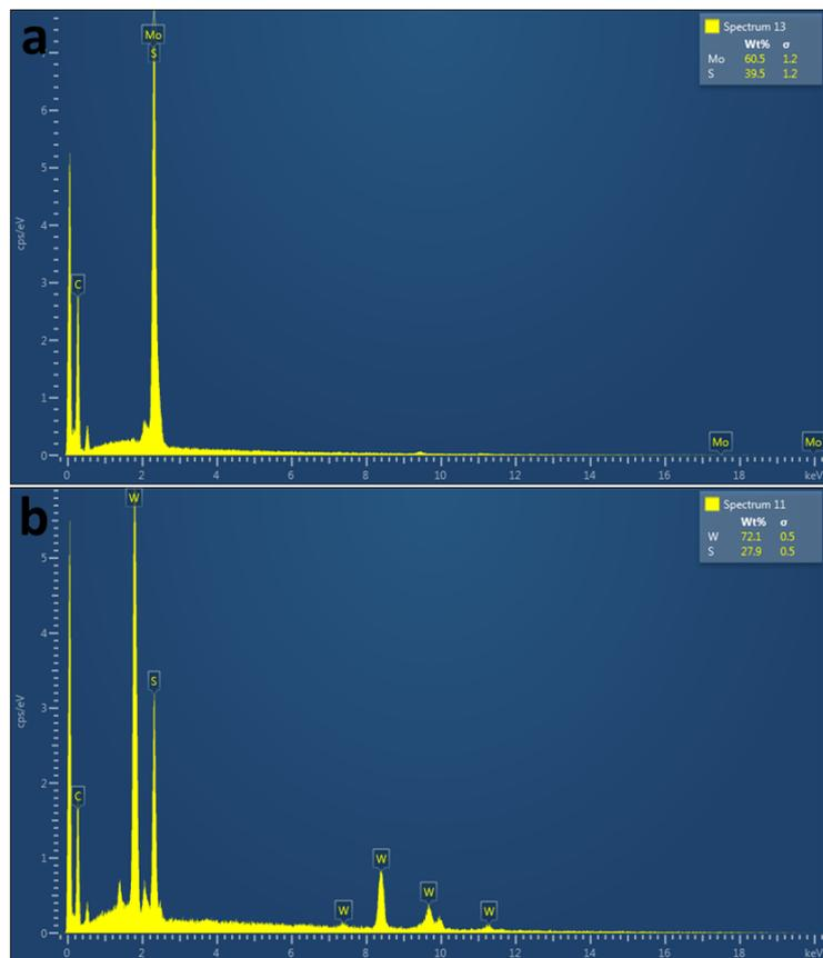
Figure S2. EDX spectrum of the nanostructured MoS<sub>2</sub>/CC and WS<sub>2</sub>/CC.
