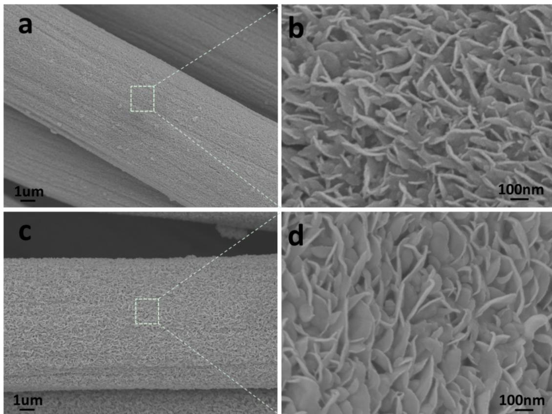
Figure S4. SEM images of the as-prepared nanostructured MoS<sub>2</sub>/CC (a&b) and WS<sub>2</sub>/CC (c&d) electrodes annealed at 350 °C for 2 h under (5%)H<sub>2</sub>/(95%)Ar.
