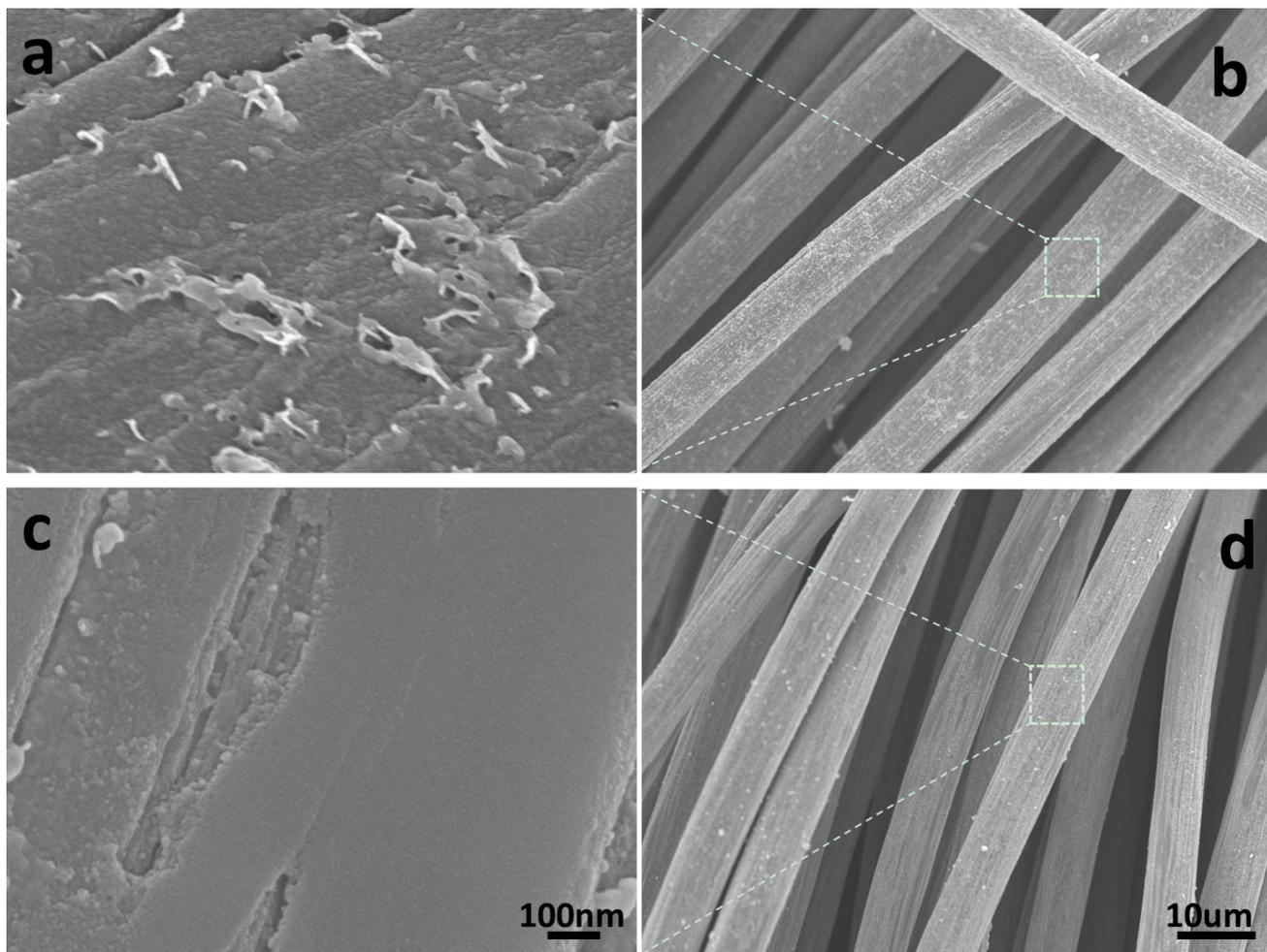
Figure S6. SEM images of flat MoS<sub>2</sub>/CC (a &b) and WS<sub>2</sub>/CC electrode (c &d).
