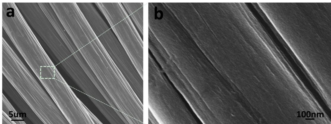
Figure S3. SEM images of carbon cloth revealing the highly textured surface of carbon microfibers.
