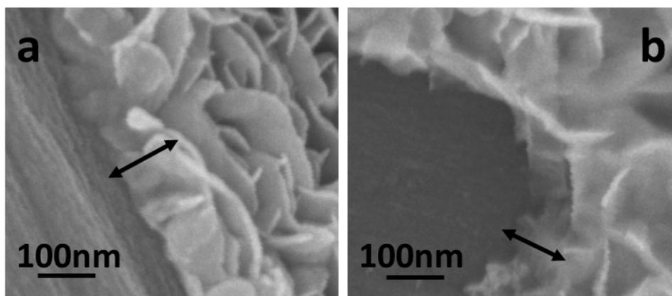
Figure S1. SEM images of the as-prepared nanostructured MoS<sub>2</sub>/CC (a) and WS<sub>2</sub>/CC (b) electrodes revealing the thickness of the films.
