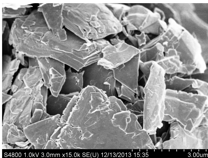
Figure S1 FESEM image of the as-prepared \text{CrO}_3 -GICs.
