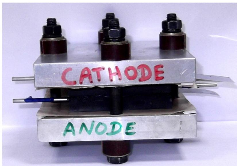
Fig S3. Photograph of polymer electrolyte membrane CO<sub>2</sub> conversion cell.
