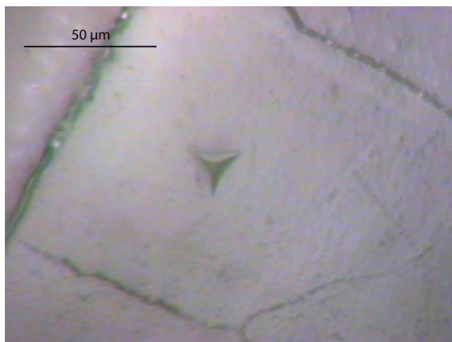
Fig. S16 1000 nm indent made on a sample (5 x 5 mm) of ZIF-8ER.
