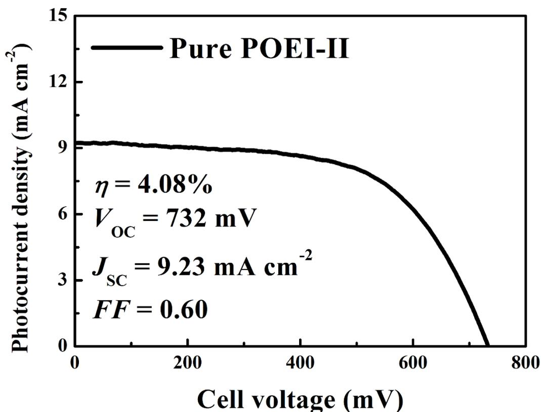
**Fig. S2.** Photocurrent density-voltage curves of the DSSCs using pure POEI-II as the electrolyte, measured at 100 mW cm<sup>-2</sup> light intensity.
