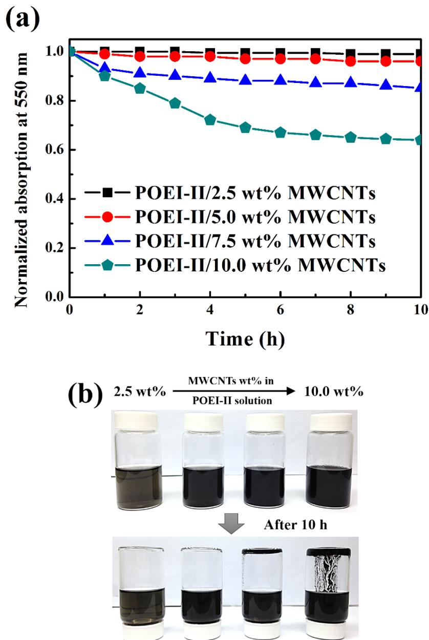
**Fig. S3.** (a) Plots of normalized absorption versus time at 550 nm for the POEI-II based ACN solutions containing different amount of MWCNTs (2.5 wt% to 10.0 wt%), and (b) the corresponding photographic images at 0 and 10 h separately.
