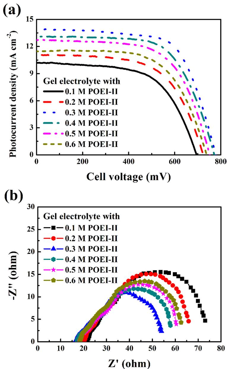
**Fig. S1.** (a) Photocurrent density-voltage curves and (b) EIS spectra of the DSSCs using the gel electrolytes containing different concentration of POEI-II, measured at  $100 \text{ mW cm}^{-2}$  light intensity.
