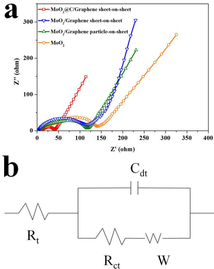
**Figure S7.** (a) Nyquist plots of the standing MoO<sub>2</sub>@C nanosheets on graphene, MoO<sub>2</sub>/Graphene sheet-on-sheet, MoO<sub>2</sub>/Graphene particle-on-sheet and MoO<sub>2</sub>@C composites, (b) Equivalent circuits.
