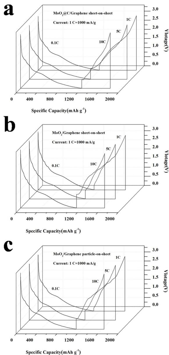
**Figure S5.** First-cycle discharge (lithium insertion) and charge (lithium extraction) curves of (a) the standing MoO<sub>2</sub>@C nanosheets on graphene, (b) the MoO<sub>2</sub>/Graphene sheet-on-sheet composite, (c) the MoO<sub>2</sub>/Graphene particle-on-sheet composite at various large current densities of 1, 5, and 10 C (1 C = 1000 mA g<sup>-1</sup>).
