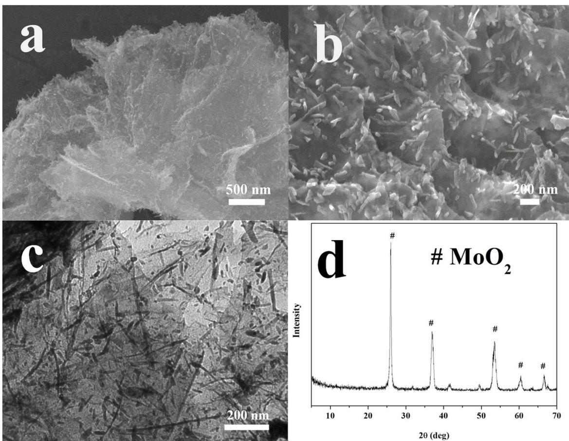
**Figure S3.** Graphene supported carbon-coated MoO<sub>2</sub> nanorods and nanoparticles: (a-b) SEM images, (c) TEM image, and (d) XRD patterns. A number of small MoO<sub>2</sub> nanorods with lengths of ~100-200 nm and diameters of ~10-20 nm are observed along with many small MoO<sub>2</sub> nanoparticles (~5-10 nm) in the composite.
