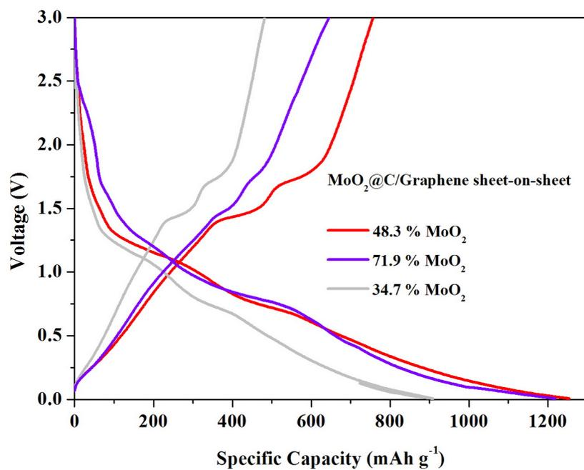
**Figure S9.** The first cycle discharge (lithium insertion) and charge (lithium extraction) curves of the MoO<sub>2</sub>@C/Graphene sheet-on-sheet composites with 34.7 %, 48.3 % and 71.9 % MoO<sub>2</sub>.
