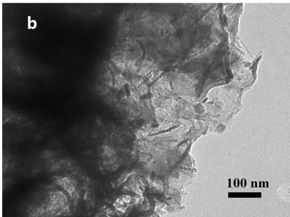
**Figure S10.** (a) XRD patterns of the cycled  $\text{MoO}_2@\text{C}/\text{Graphene}$  (48.3 %  $\text{MoO}_2$ ). The crystalline  $\text{MoO}_2$  is changed to be amorphous after repetitive 100 cycles. (b) TEM image of the cycled composite electrode after 100 cycles. The cross-section of the standing  $\text{MoO}_2$  nanosheets can be still observed on graphene although there is a presence of a large amount of PVDF binder and carbon black in the electrode.
