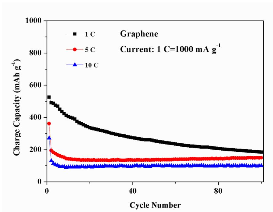
**Figure S6.** High-rate cycling performances of bare graphene. Initial charge (lithium extraction) capacities of bare graphene were 526, 362, and 272 mAh/g at 1 C, 2 C, and 5 C respectively, which decreased to 231, 150, 101 mAh/g after 100 cycles.
