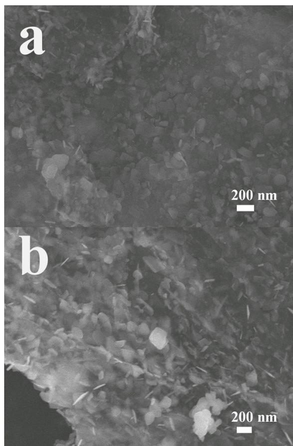
**Figure S4.** SEM images of the standing MoO<sub>2</sub>@C nanosheets on graphene. (a) reaction time: 0.5 h, (b) reaction time: 1 h. It seems that MoO<sub>2</sub>@C nanosheets are not formed completely compared to the main product after 2 h as shown in Figure 3 of main text. These tattered nanosheets exhibit smaller size of ~100-150 nm after shorter reaction time.
