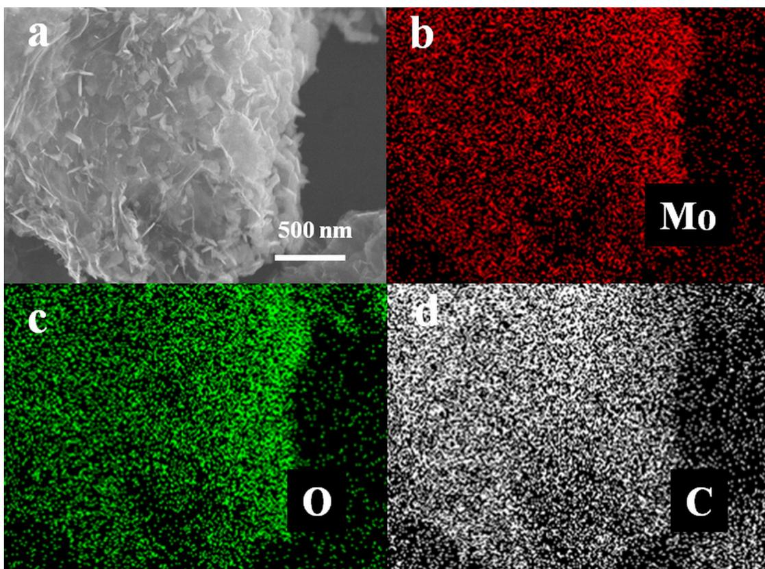
**Figure S2.** Elemental mapping images of the standing  $\text{MoO}_2@\text{C}$  nanosheets on graphene (48.3 %  $\text{MoO}_2$ ). Mo, O, and C elements are also distributed uniformly in the composite.
