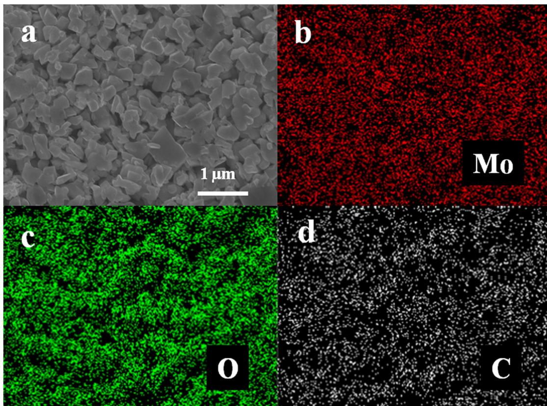
**Figure S1.** Elemental mapping images of the  $\text{MoO}_2@\text{C}$  composite. Mo, O, and C elements are distributed uniformly in the product. It is confirmed that carbon is formed around  $\text{MoO}_2$  by acetylene decomposition.
