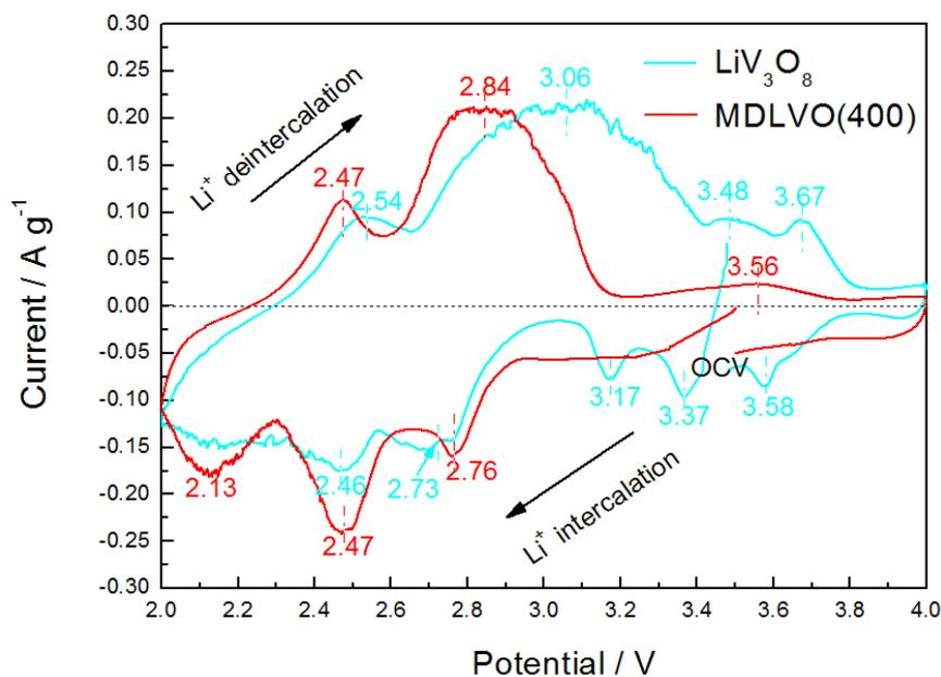
Figure S6 The first-cycle CV curves for pure  $\text{LiV}_3\text{O}_8$  calcined at  $400^\circ\text{C}$  and Mo-doped  $\text{LiV}_3\text{O}_8$  (400) electrodes at a scan rate of  $0.1 \text{ mV s}^{-1}$  over the range of 2.0-4.0 V (vs.  $\text{Li}/\text{Li}^+$ ).
