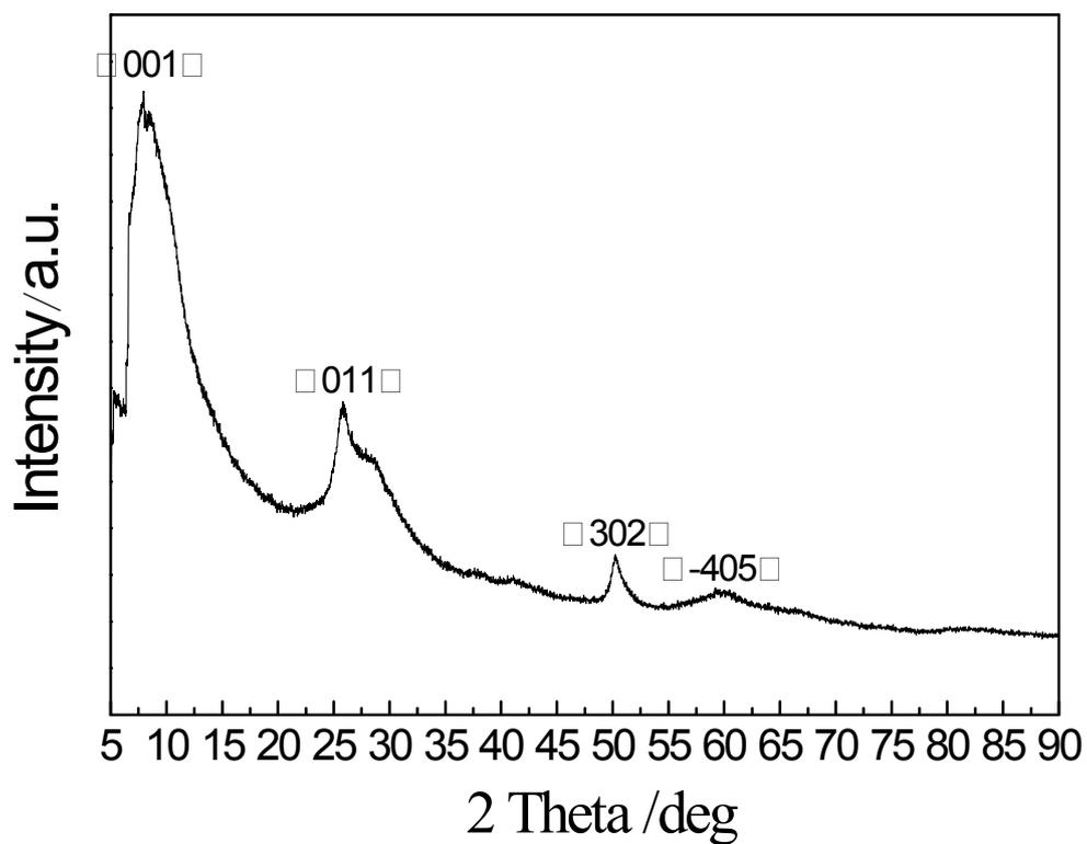
Figure S4 XRD pattern of milled Mo-doped  $\text{LiV}_3\text{O}_8$  cryogel obtained by freeze drying.
