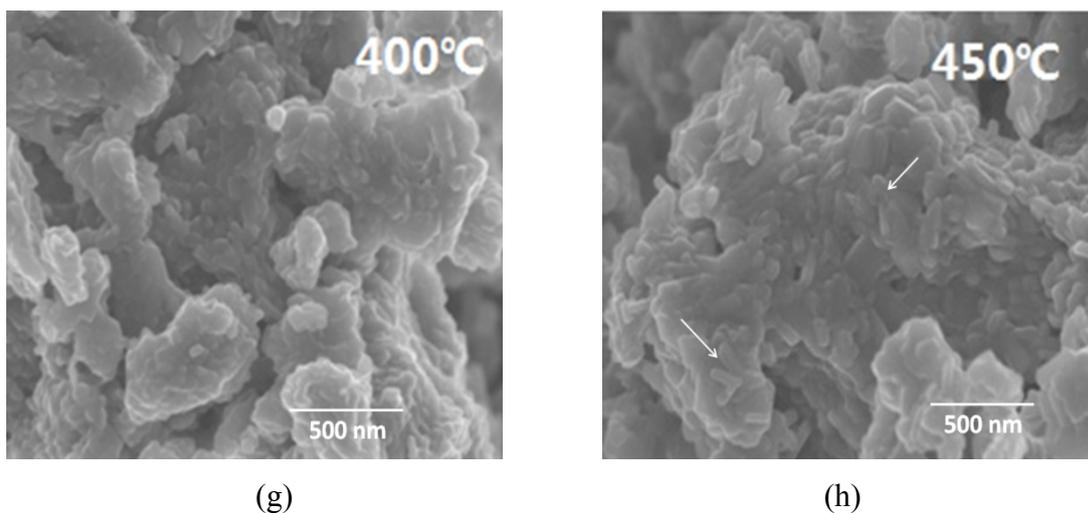
Figure S3 FE-SEM images of Mo-doped  $\text{LiV}_3\text{O}_8$  cryogel (a, b), Mo-doped  $\text{LiV}_3\text{O}_8$  calcined at  $400^\circ\text{C}$  (c, d) and milled Mo-doped  $\text{LiV}_3\text{O}_8$  calcined at  $300^\circ\text{C}$  (e),  $350^\circ\text{C}$  (f),  $400^\circ\text{C}$  (g) and  $450^\circ\text{C}$  (h).
