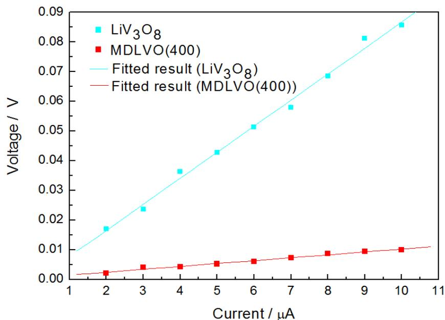
Figure S2 Current-voltage curves obtained by the DC four-probe measurements for  $\text{LiV}_3\text{O}_8$  calcined at  $400^\circ\text{C}$  and Mo-doped  $\text{LiV}_3\text{O}_8$  (400) samples at room temperature.
