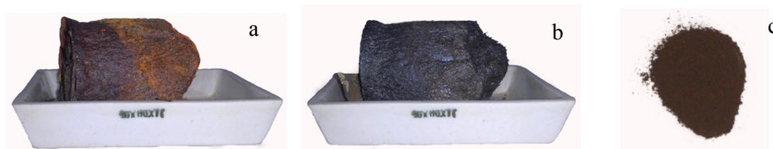
Figure S1 (a) Mo-doped  $\text{LiV}_3\text{O}_8$  cryogel obtained by freeze drying. (b) Mo-doped  $\text{LiV}_3\text{O}_8$  nanorod-assembled sheets obtained by annealing the cryogel in ambient atmosphere at  $400^\circ\text{C}$  for 2 h. (c) Mo-doped  $\text{LiV}_3\text{O}_8$  nanorod-assembled nanosheets obtained after ball milling.
