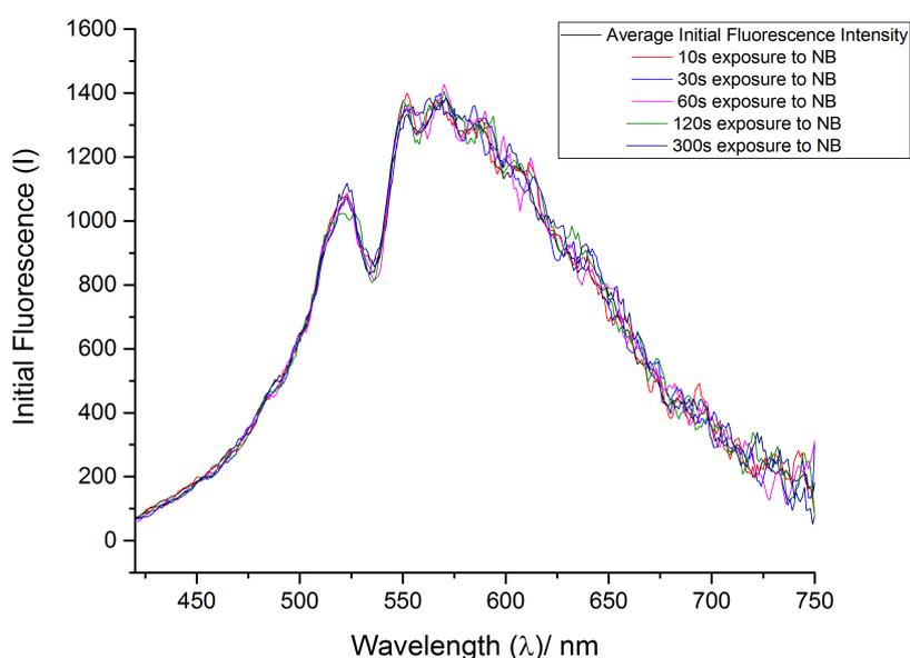
S6.1 - Fluorescence emission profile of the free linker ligand H<sub>2</sub>dc bpy upon exposure to NB.
