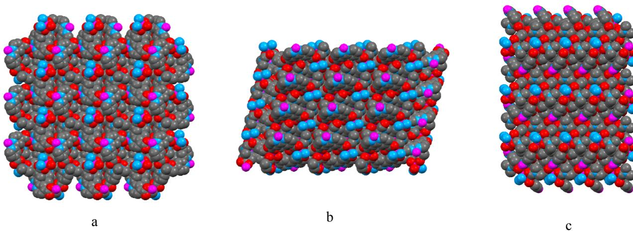
Figure S2.2 shows the space filling diagrams of MOF **1'** with views along the crystallographic a) *a*-axis, b) *b*-axis and c) *c*-axis.
