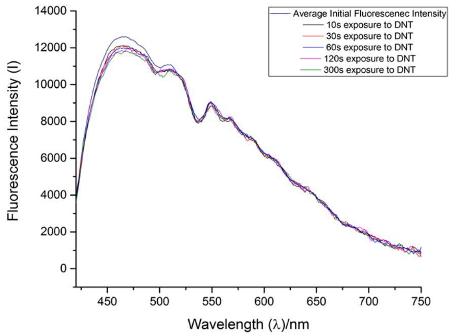
**Figure 6.4** – Fluorescence emission profiles of MOF **1M'** thin films upon exposure to analytes DMNB, NB, p-NT and 2,4-DNT.
