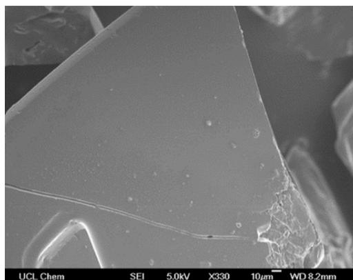
**Figure S3.2** – An SEM of a typical MOF 1' thin film
