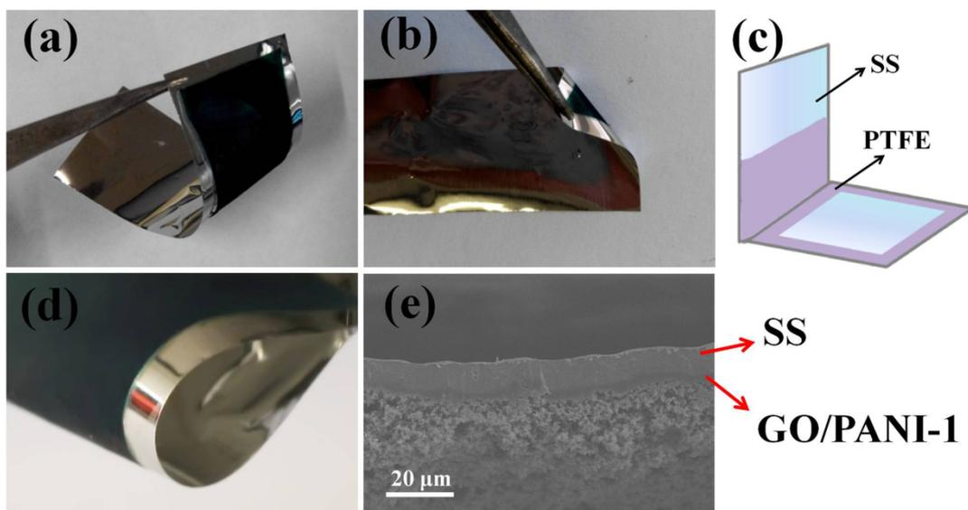
**Fig. S1** Optical images of (a) one side (contact with water) and (b) the other side (contact with chloroform) of the electrode by interfacial electrochemical polymerization. (c) Scheme of the bended SS foil with Teflon layer cover. (d) The enlarged image of the bended electrode. (e) SEM image of the electrode at the cross-section.
