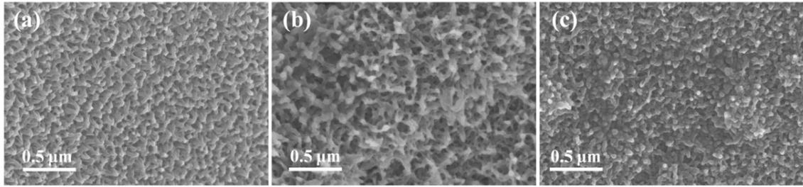
**Fig. S4** SEM image of GO/PANI-1 prepared at the concentration of aniline (a) 0.05M, (b) 0.1M and (c) 0.5 M.
