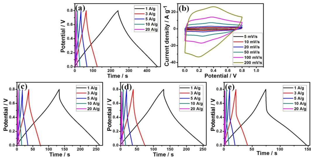
**Fig. S7** (a) Galvanostatic charge-discharge curves of the GO/PANI-1 supercapacitor at different current densities. (b) CV curves of GO/PANI-1 supercapacitor at different scan rates. Galvanostatic charge-discharge curves of supercapacitors based on (c) GO/PANI-2, (d) PANI-1 and (e) PANI-2 at different current densities.
