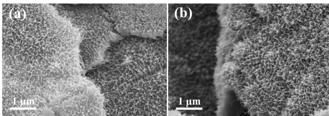
**Fig. S2** SEM images of GO/PANI on two different electrodes under the same polymerization condition.
