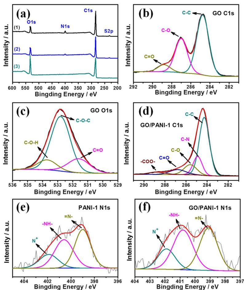
**Fig. S5** (a) XPS spectra of (1) PANI-1, (2) GO/PANI-1 and (3) GO. (b) C 1s spectrum of GO. (c) O 1s spectrum of GO. (d) C 1s spectrum of GO/PANI-1. (e) and (f) N 1s spectrum of PANI-1 and GO/PANI-1, respectively.
