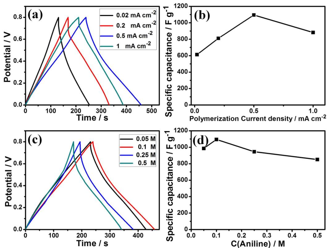
**Fig. S6** (a) galvanostatic charge-discharge curves and (b) mass specific capacitance of GO/PANI-1 nanocomposites at various current densities of polymerization (0.02, 0.2, 0.5, 1 mA cm<sup>-2</sup>), (c) galvanostatic charge/discharge curves and (d) mass specific capacitance of GO/PANI-1 nanocomposites at various concentrations of aniline (0.05, 0.1, 0.25, 0.5 M).
