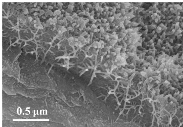
**Fig. S9** A high-resolution SEM image of GO/PANI-1 showing a well contact between GO and PANI.
