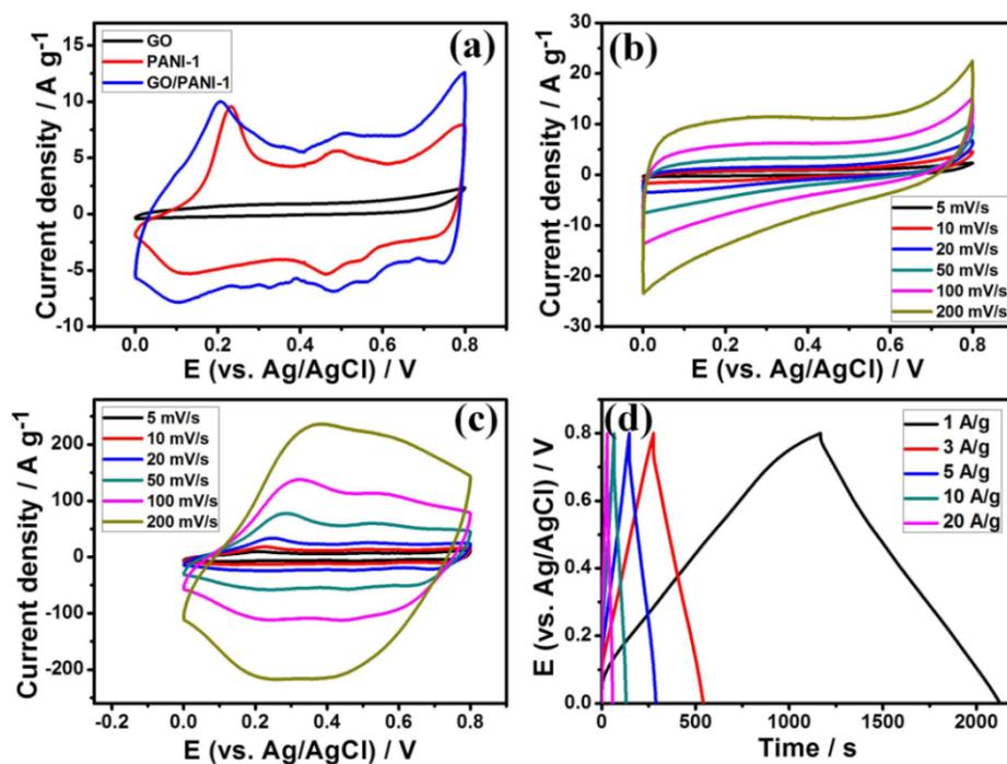
**Fig. S8** (a) CV curves of GO, PANI-1 and GO/PANI-1 nanocomposite at 5 mV s<sup>-1</sup>. (b) and (c) CV curves of GO and GO/PANI-1 nanocomposite at different scan rates. (d) Galvanostatic charge-discharge curves of GO/PANI-1 nanocomposite at different current densities.
