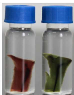
Figure S4. Photographs of PEG-HDI 1.2 -TPP hydrogels in Tris-HClO 4 buffer solution (left) and in Hg 2+ solution (10 mM, right), pH values of these solution are all 7.0, controlled by the Tris-HClO 4 buffer solution.
