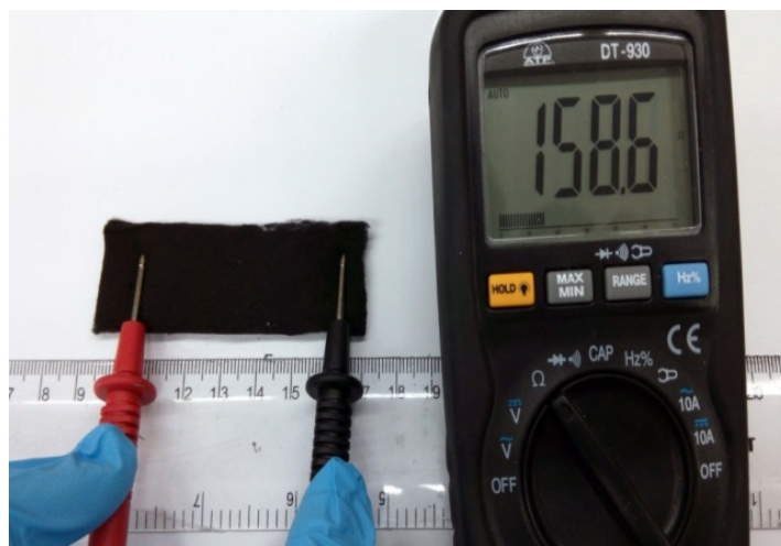
Figure S2. Photograph shows the low resistance of CC ( 158.6 \Omega ).
