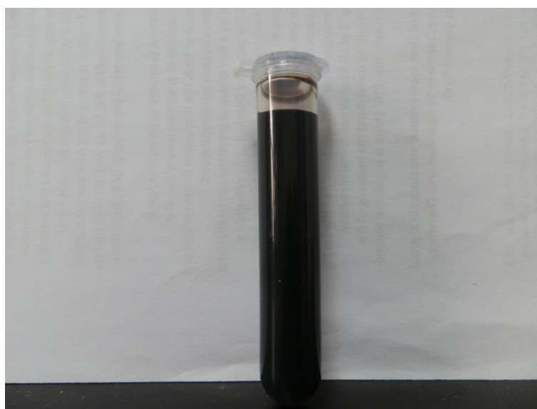
Fig. S2 The upper solution after centrifugation. The synthesis condition: F127: 3.8 mM. 3-Aminophenol, 10 mmol; HMT, 5 mmol; ammonia concentrations: 0.37 M.
