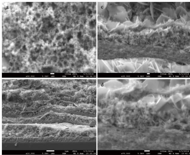
**Figure S4.**  $\text{Bi}_2\text{S}_3/\text{rGO}$  multilayer on  $\text{TiO}_2$  nanoparticles thin film.
