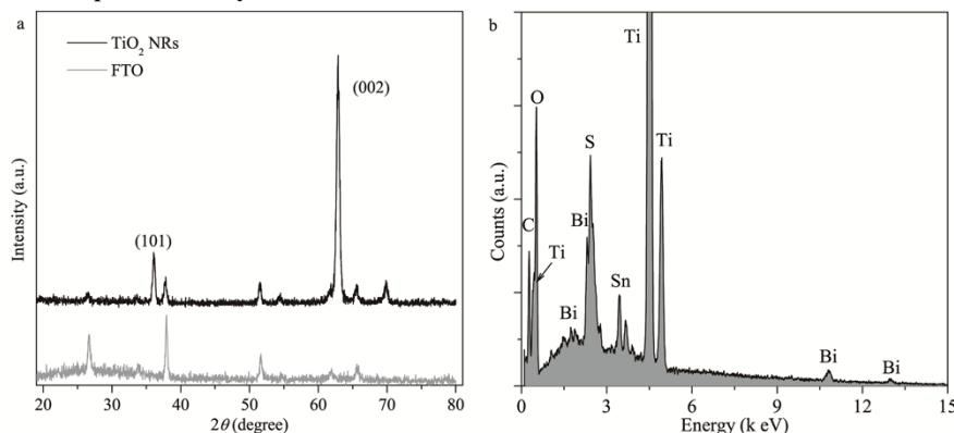
**Figure S5.** a. XRD pattern of  $\text{TiO}_2$  NRs on FTO substrates. b. Typical EDS pattern of  $(\text{Bi}_2\text{S}_3/\text{rGO})_5/\text{TiO}_2$  NRs electrodes.
