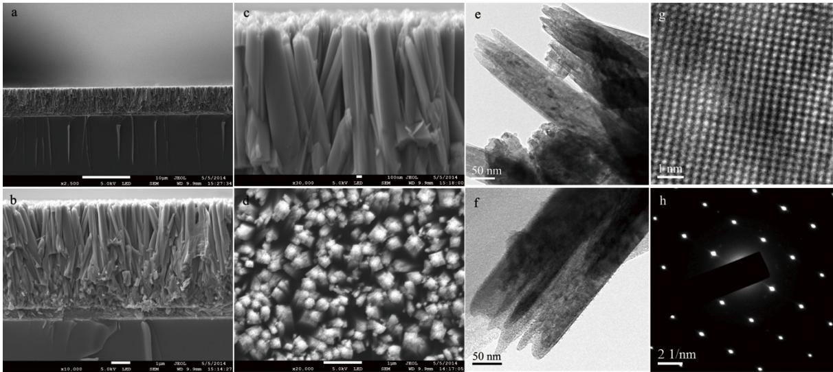
**Figure S1.**  $\text{TiO}_2$  nanorod arrays (NRs) on FTO substrates.
