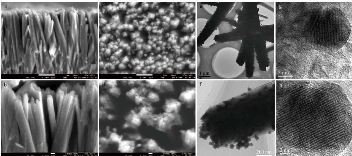
**Figure S2.**  $\text{Bi}_2\text{S}_3$  nanoparticles decorated  $\text{TiO}_2$  NRs on FTO substrates.
