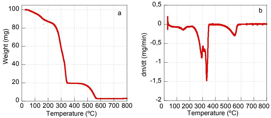
**Figure S12:** TGA heating curve of **Ss1** (a) and its 1<sup>st</sup> derivative peaks (b).
