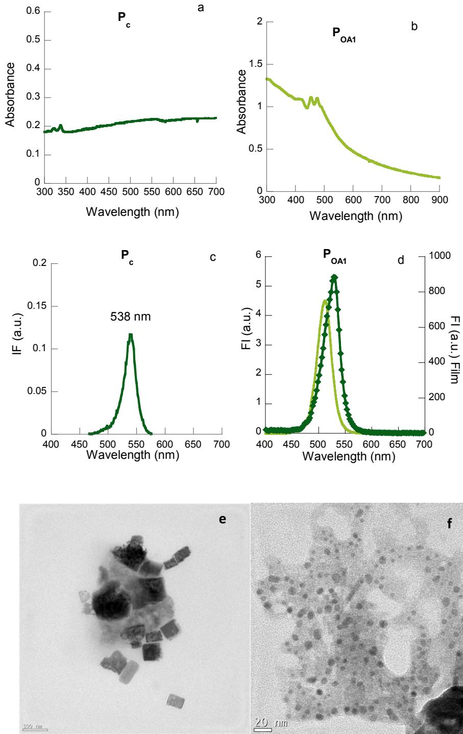
**Figure S1:** Absorption spectra of **Pc** (a) and **PoA1** (b) in toluene. Emission spectra of **Pc** (c) and **PoA1** in toluene (light green) (d); and **PoA1** film (dark green) (d). Emission recorded at  $\lambda_{\text{exc}} = 350$  nm. (d) HRTEM images (scale bar 20 nm) of **Pc** (e) and **PoA1** (f).
