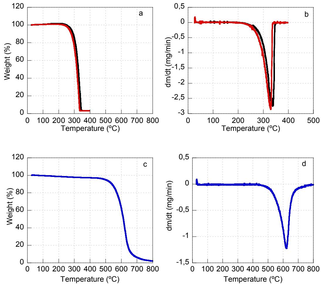
**Figure S9:** TGA heating curve of MABr and OABr (a, black and red, respectively) and of PbBr<sub>2</sub> (c); 1<sup>st</sup> derivative peaks of MABr and OABr (b, black and red, respectively) and of PbBr<sub>2</sub> (d).
