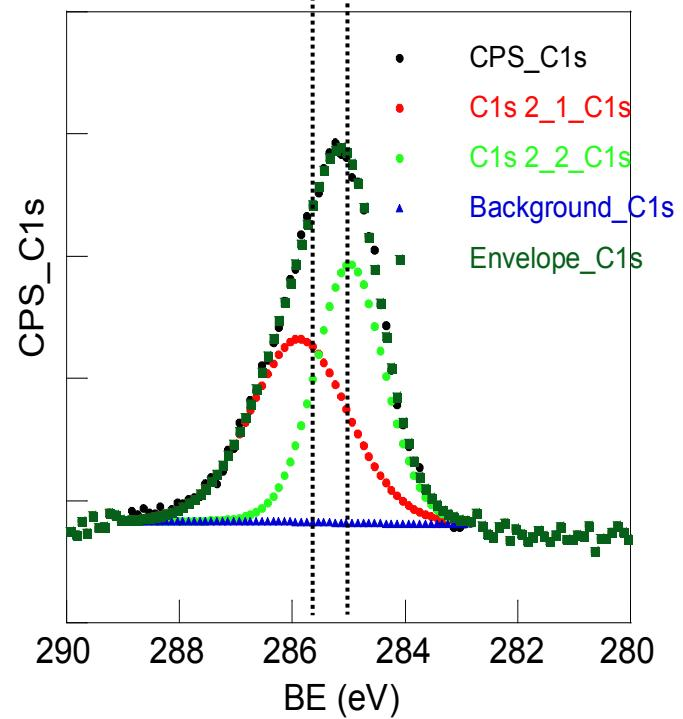
**Figure S4:** XPS spectra of C1s for  $P_{OA1}$  (a) and  $P_{OA2}$  (b)
