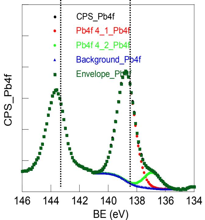
**Figure S7:** XPS spectra of Pb4f for  $P_{OA1}$  (a) and  $P_{OA2}$  (b)
