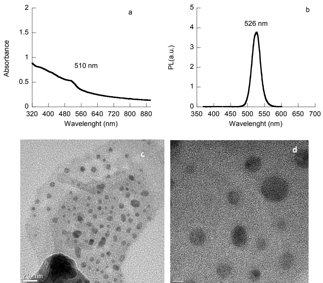
**Figure S3:** Absorption and emission spectra of  $\text{P}_{\text{HA}}$  (a, b) in toluene; emission recorded at  $\lambda_{\text{exc}} = 350 \text{ nm}$ , and HRTEM images with a scale bar of 20 (c) and 5 nm (d). Size  $5.92 \pm 2.05 \text{ nm}$
