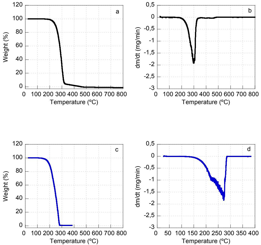
**Figure S10:** TGA heating curve of OLA and ODE (a and c, in black and blue, respectively) and its 1<sup>st</sup> derivative peaks (b and d).
