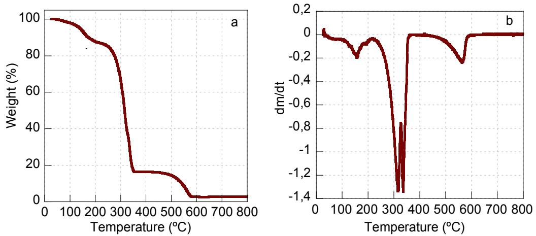
**Figure S13:** TGA heating curve of **Ss2** (a) and its 1<sup>st</sup> derivative peaks (b).
