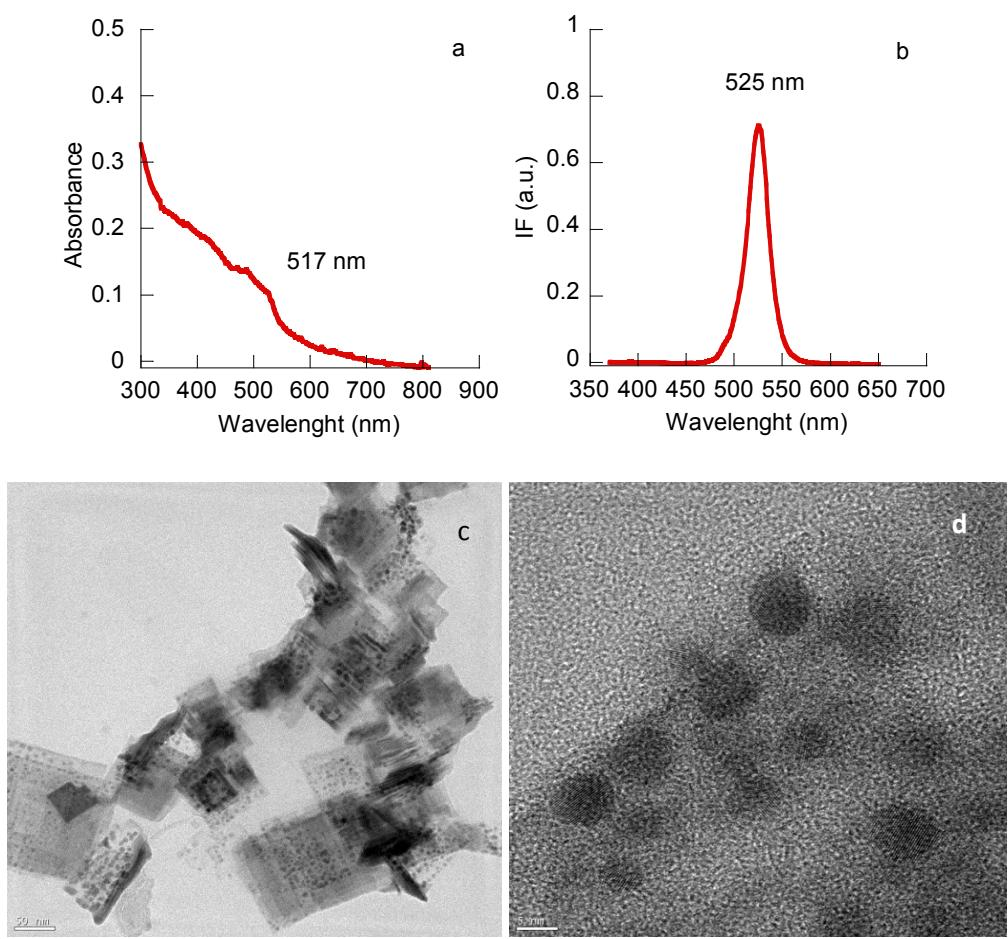
**Figure S2:** Absorption (a) and emission (b) spectra of  $\text{P}_{\text{O}\text{A}3}$  in toluene; emission recorded at  $\lambda_{\text{exc}} = 350$  nm. (c) and (d) HRTEM images at 50 and 5 nm scale, respectively. Nanoparticle size  $5.92 \pm 1.79$  nm.
