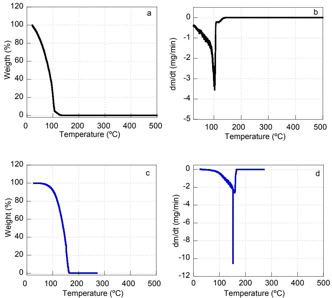
**Figure S11:** TGA heating curve of MA and OA (a and c, in black and blue, respectively) and its 1<sup>st</sup> derivative peaks (b and d).
