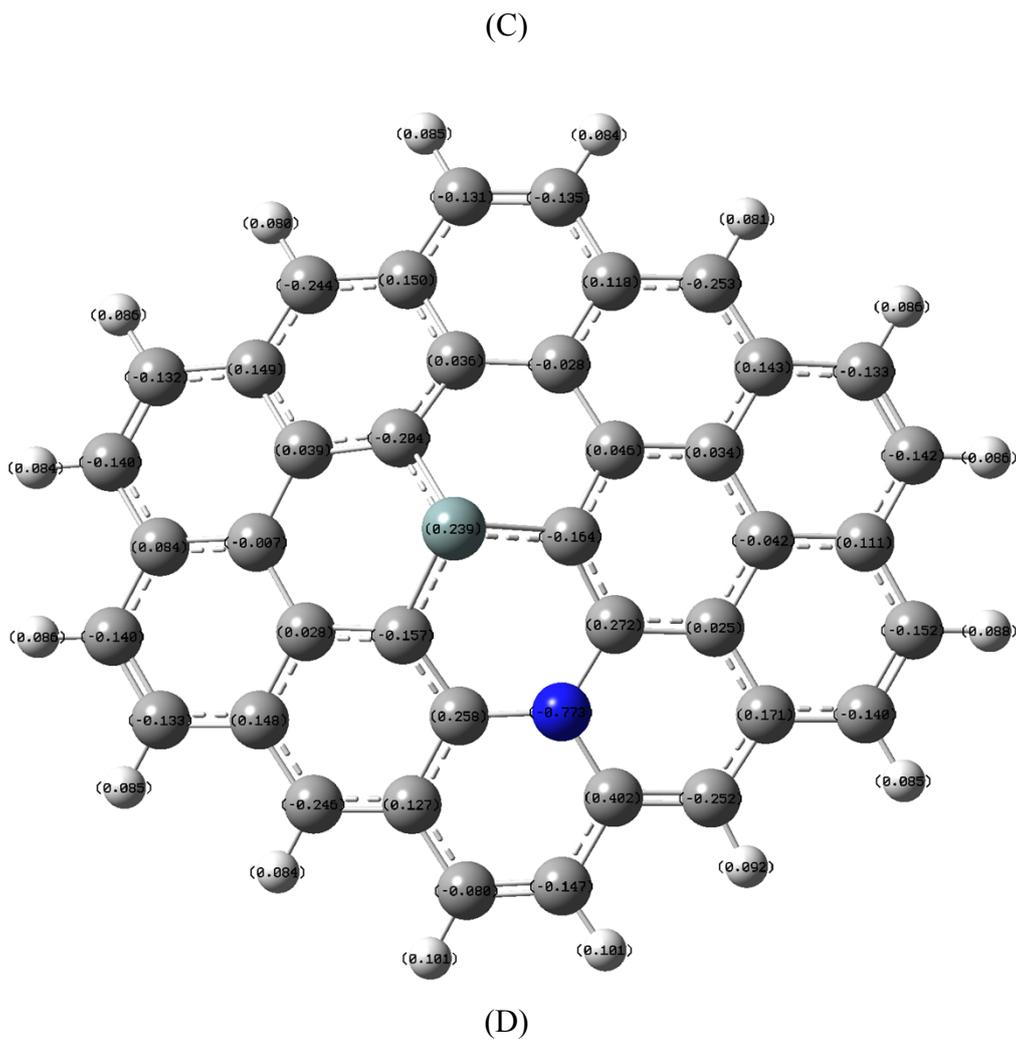
Fig. S3. The net charge distributions of C, Si and N atoms in pure graphene (A), Si-doped graphene with one silicon (B) or two silicon atoms (C) and Si, N-codoped graphene (D).
