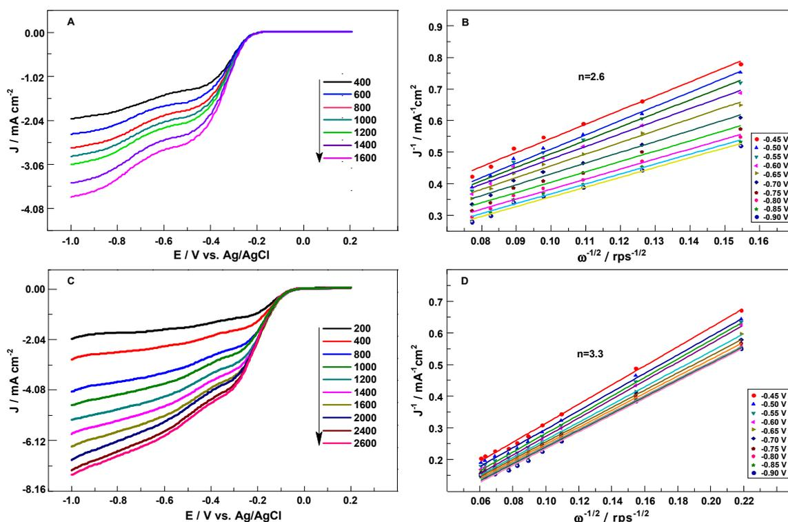
Fig. S2 Koutecky-Levich plots of  $J^{-1}$  versus  $\omega^{-1/2}$  at different electrode potentials of SiN-CNTs (A, B) and Si-CNSs (C, D) obtained from the LSVs at different rotating speeds from 200 rpm to 2600 rpm.
