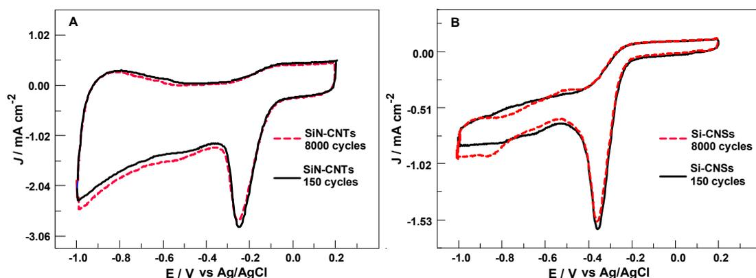
Fig. S1. The CVs of the 150<sup>th</sup> and 8000<sup>th</sup> cycles of the SiN-CNTs (A) and Si-CNSs (B) in an oxygen-saturated 0.1 M KOH solution in the three-electrode system with a graphite
