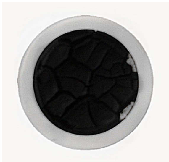
Figure S3. Fabrication of Fe 3 O 4 /RGO hybrids with 50 wt% Fe 3 O 4 .
