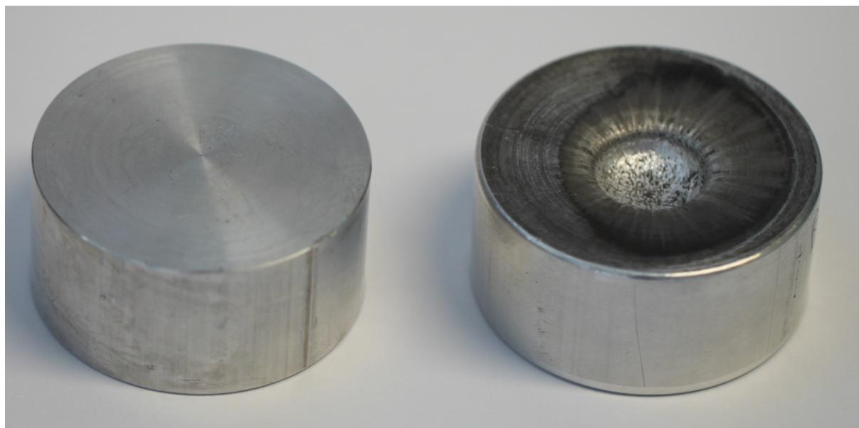
**Figure S9.** Aluminum block of the SSRT before (left) and after (right) detonation of dinitramide **2**.
