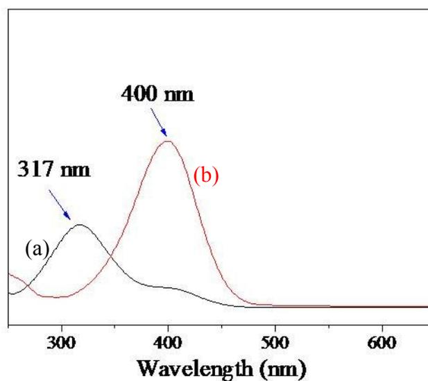
Figure S5 UV-vis absorption spectra of 4-NP (a) without and (b) with the addition of NaBH<sub>4</sub> solution.
