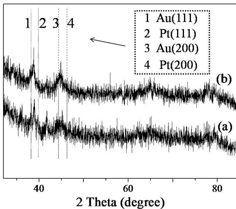
Figure S3 XRD patterns for the SiO<sub>2</sub>/AuPt with different ratio of AuPt dosage. (a) 0.5:1, and (b) 1:1(The corresponding TEM images were shown in Figure S8a). All the samples were sequentially suffered from roasting under air and then H<sub>2</sub> atmosphere.
