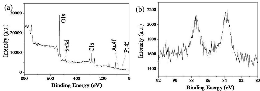
Figure S4 XPS spectra of the Fe@SiO<sub>2</sub>/AuPt nanocomposites: (a) fully scanned spectra, and (b) Au 4f spectra.
