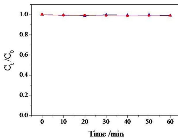
Figure S6  $C_t/C_0$  versus reaction time for the reduction of 4-NP with Fe@SiO<sub>2</sub> NCs (blue line), and Fe@SiO<sub>2</sub>-Sn NCs (red line).
