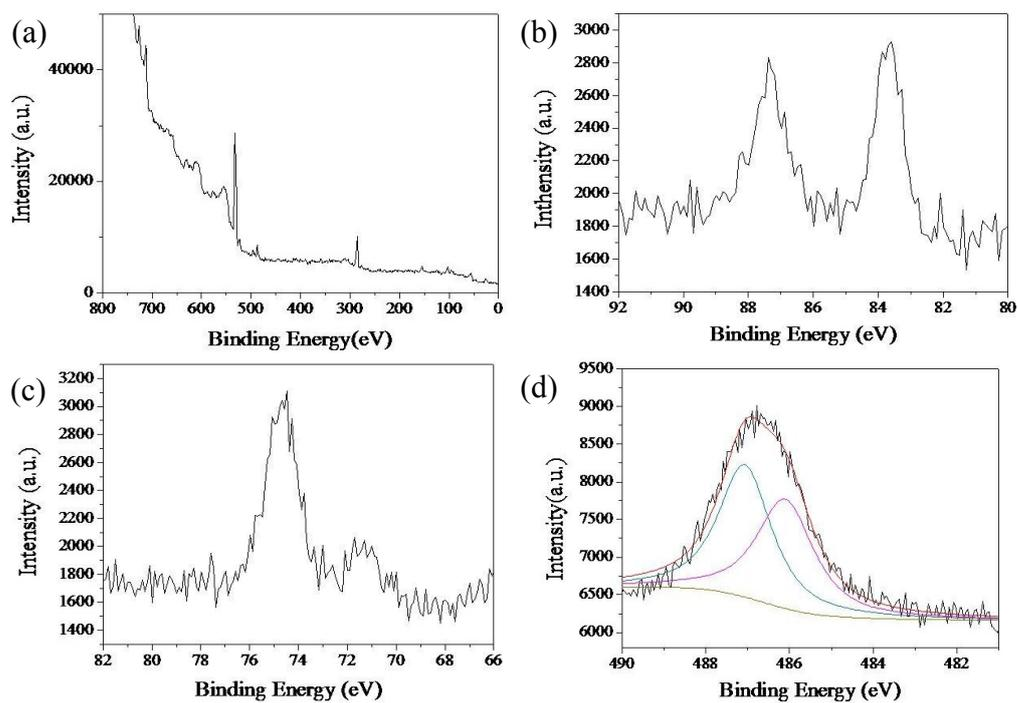
Figure S7 XPS spectra of the Fe/SiO<sub>2</sub>/AuPt composites after reduction reaction of 4-NP. (a) Fully scanned spectra, (b) Au 4f spectra, (c) Pt 4f spectra, and (d) Sn 3d spectra.
