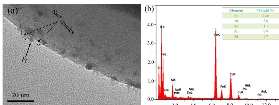
Figure S1 (a) Representative enlarged TEM image of Fe<sub>2</sub>O<sub>3</sub>@SiO<sub>2</sub>/Pt to show the “islands in the sea” configuration (one side of Pt NPs linking with SiO<sub>2</sub> layer is covered with a smooth layer and another side of Pt NPs is exposed). (b) EDX spectroscopy of the as-prepared Fe<sub>2</sub>O<sub>3</sub>@SiO<sub>2</sub>/AuPt NPs and the corresponding element composition.
