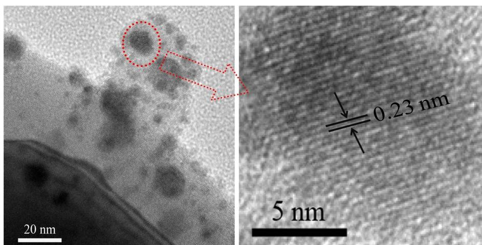
Figure S2 A representative HRTEM image of AuPt NPs on the surface of Fe@SiO<sub>2</sub> NCs.
