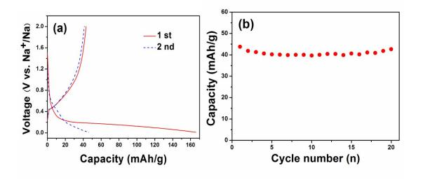
**Figure S1** (a) The initial two discharge/charge profiles of the pyrolyzed carbon electrode between 0.01 V and 2.0 V vs. Na<sup>+</sup>/Na at a current rate of 100 mA g<sup>-1</sup>; (b) Cycling performance of the pyrolyzed carbon electrode at a current rate of 100 mA g<sup>-1</sup>.
