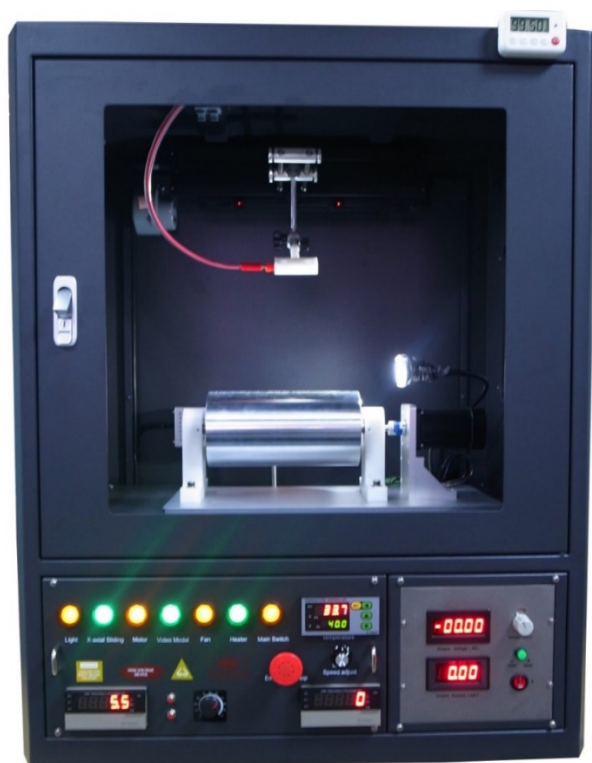
Figure S8. The photograph of electrospinning equipment (TL01, Shenzhen TONGLI Micro & Nano Tech. LTD.)
