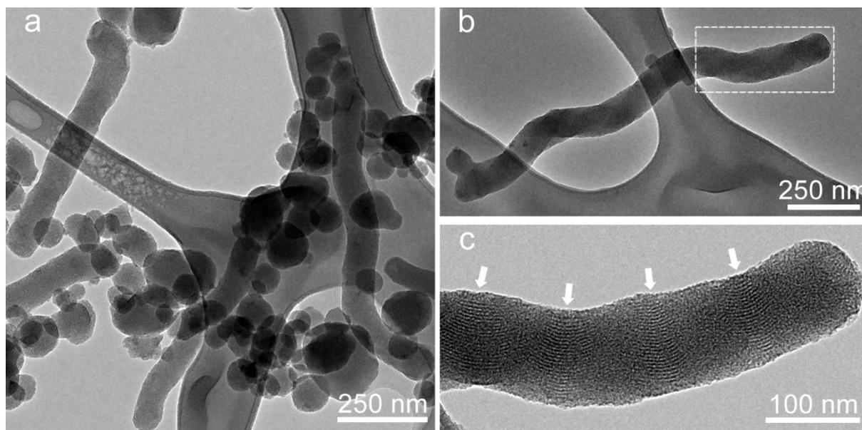
**Fig. S1** TEM images of MSNs prepared using 20 mg of RB. (a) Low magnification image showing the polydispersity of the particles. (b) TEM image of a helical nanorod with large aspect ratio. (c) Close-up image of the helical nanorod shown in (b). White arrows indicate the helical porous structure of the nanorod.
