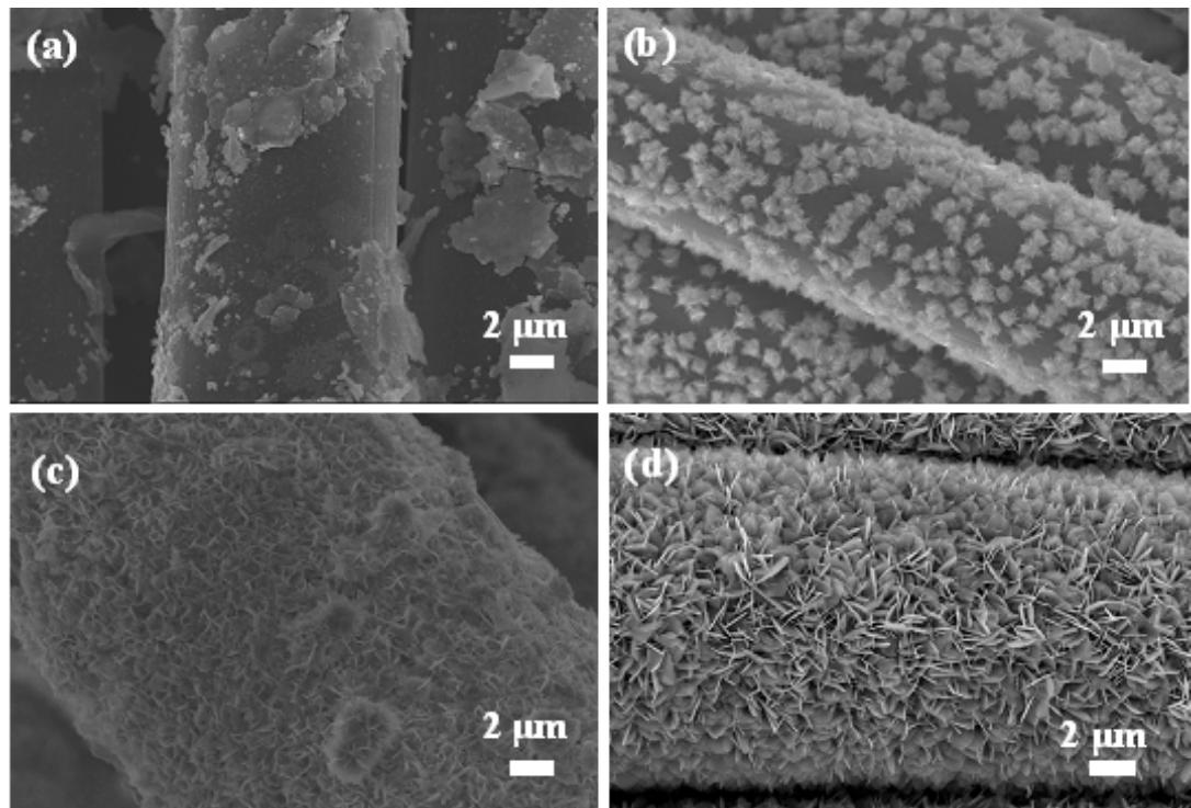
Figure S1. SEM images of hierarchical SnO<sub>2</sub> nanostructures with different reaction time (a) 2 h, (b) 4 h, (c) 6 h, (d) 8 h.
