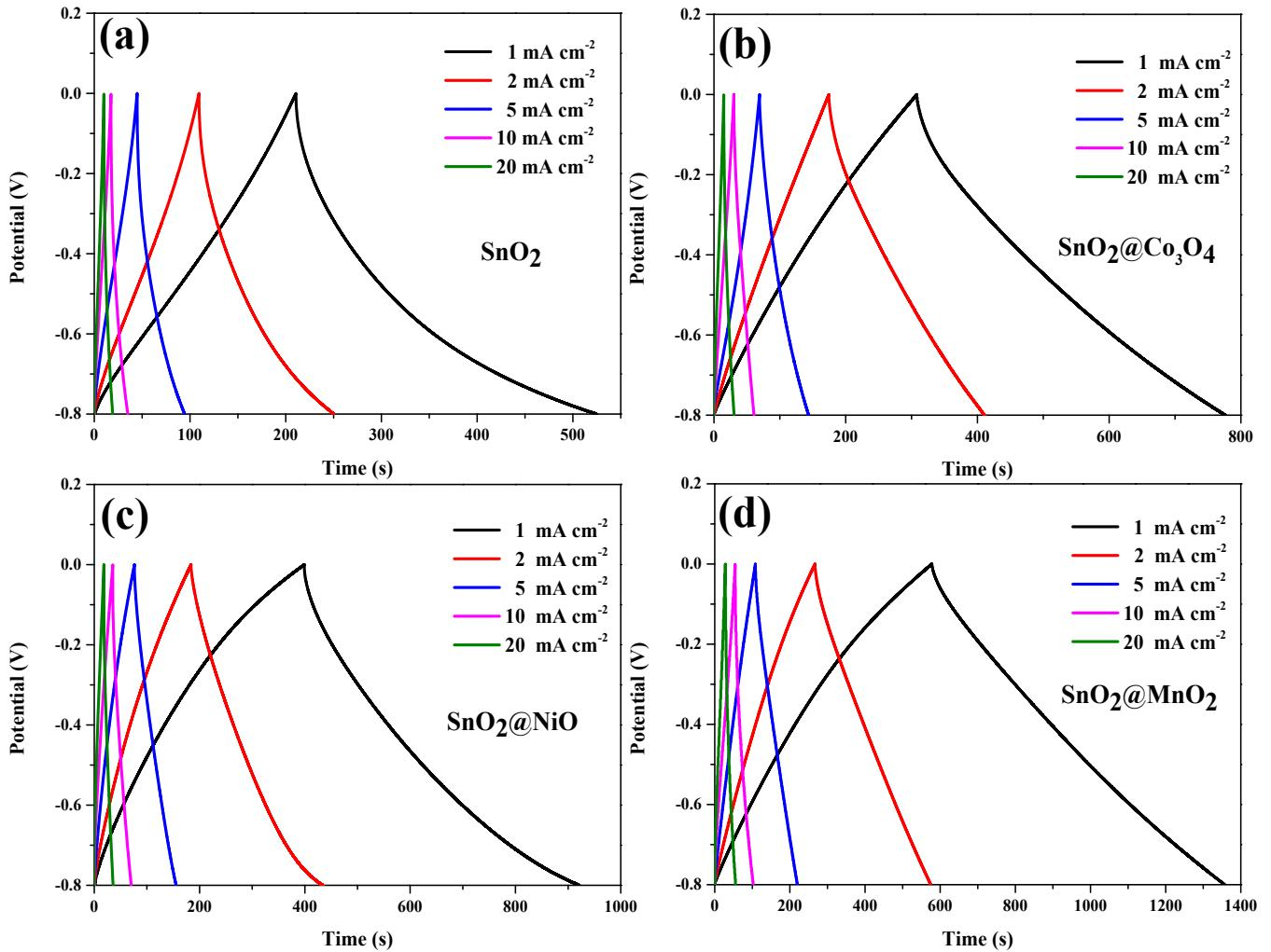
Figure S4. Charge and discharge curves of (a) SnO<sub>2</sub>, (b) SnO<sub>2</sub>@Co<sub>3</sub>O<sub>4</sub>, (c) SnO<sub>2</sub>@NiO, (d) SnO<sub>2</sub>@MnO<sub>2</sub> at different current density of 1, 2, 5, 10 and 20 mA cm<sup>-2</sup>.
