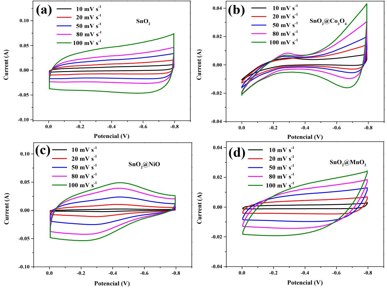
Figure S3. Cyclic voltammetry curves of (a)  $\text{SnO}_2$ , (b)  $\text{SnO}_2@\text{Co}_3\text{O}_4$ , (c)  $\text{SnO}_2@\text{NiO}$ , (d)  $\text{SnO}_2@\text{MnO}_2$  at different scan rates of 10, 20, 50, 80 and 100  $\text{mV s}^{-1}$  in 1M  $\text{Na}_2\text{SO}_4$  aqueous solution, respectively.
