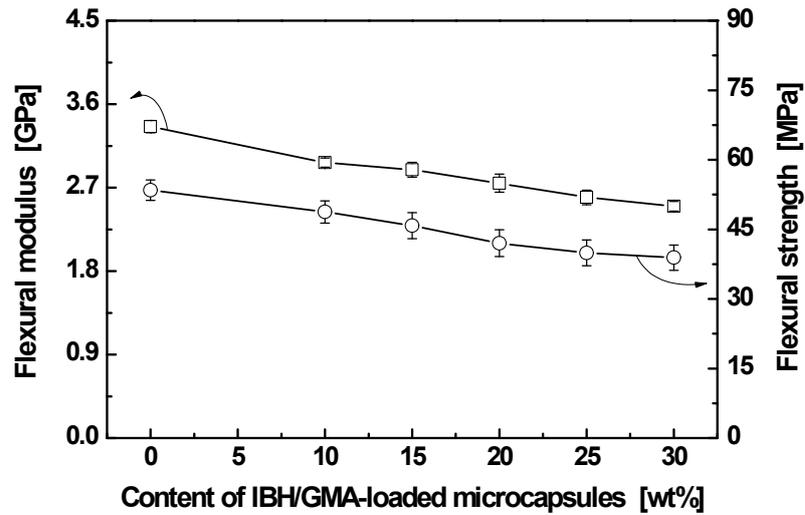
**Figure S6.** Dependences of flexural modulus and strength of authentic self-healing PS composite on content of IBH/GMA-loaded microcapsules. 3 wt% NaBH<sub>4</sub> particles were embedded in PS, while the IBH concentration in IBH/GMA was 2 wt%. Flexural modulus and strength of unfilled PS are 3.35 GPa and 53.5 MPa, respectively.
