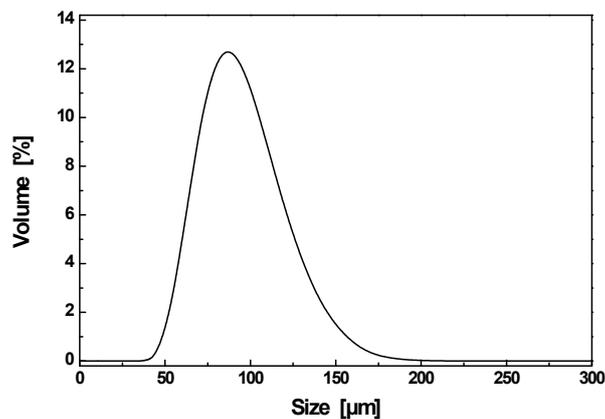
**Figure S2.** Size distribution of IBH/GMA solution-loaded microcapsules used for making the self-healing PS composites investigated in this paper. Concentration of IBH in the IBH/GMA solution: 2 wt%.
