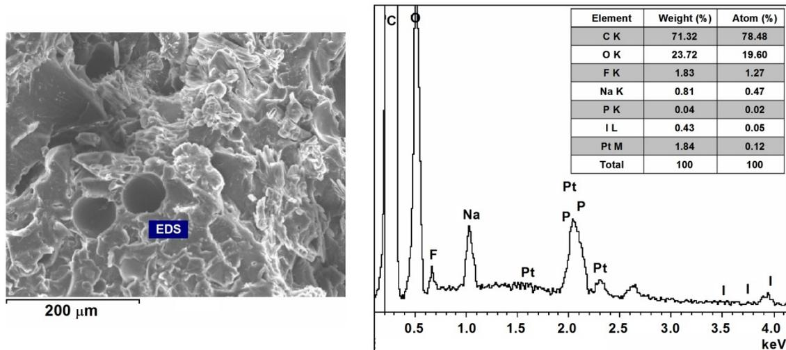
**Figure S8.** EDS analysis of the re-fractured surface of a healed self-healing PS composite specimen containing 20 wt% IBH/GMA solution-loaded microcapsules and 3 wt% NaBH<sub>4</sub> particles.
