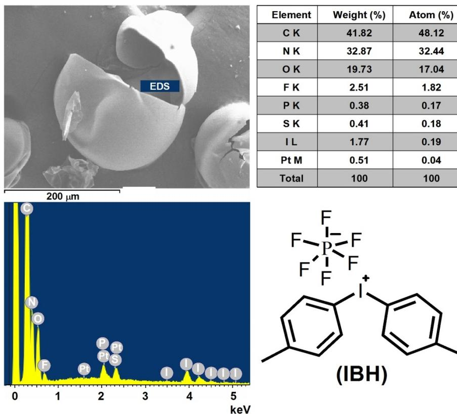
**Figure S3.** EDS analysis of IBH/GMA solution-loaded microcapsules.
