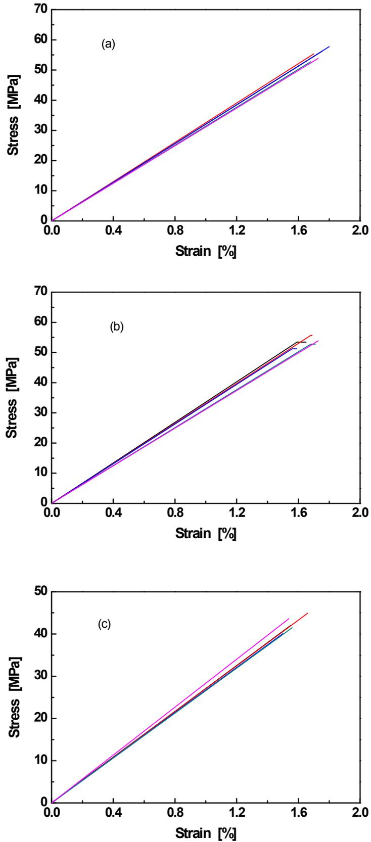
**Figure S5.** Flexural stress-strain curves of a) PS, b) PS composite containing 3 wt% NaBH<sub>4</sub>, and c) PS composite containing 3 wt% NaBH<sub>4</sub> and 20 wt% IBH/GMA-loaded microcapsules.
