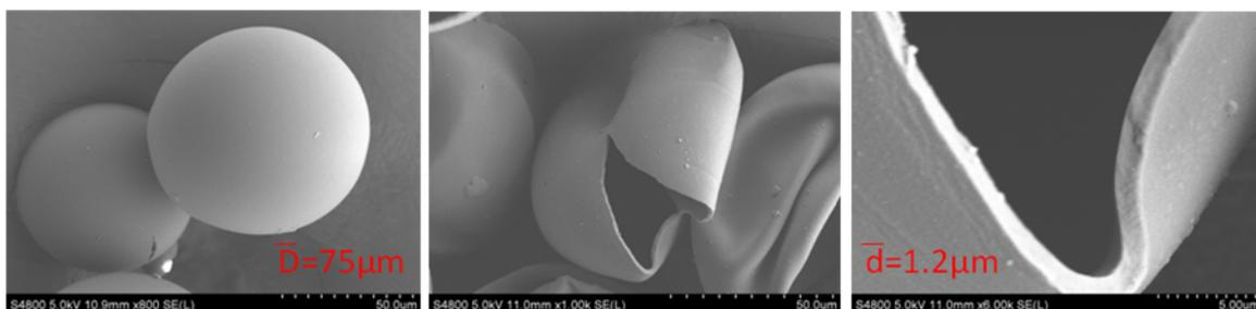
**Figure S1.** SEM micrographs of IBH/GMA solution-loaded microcapsules showing the full view and shell thickness. Concentration of IBH in the IBH/GMA solution: 2 wt%.
