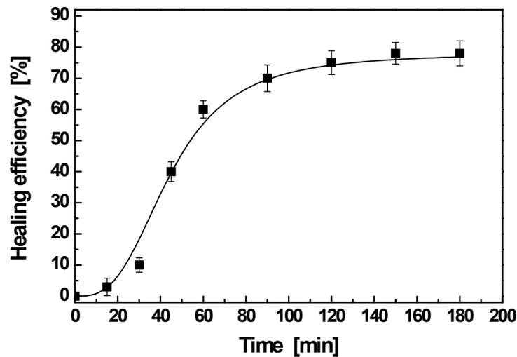
**Figure S7.** Dependence of healing efficiency of authentic self-healing PS composite on healing time. The composite is filled with 20 wt% IBH/GMA-loaded microcapsules and 3 wt% NaBH<sub>4</sub> particles (IBH concentration in IBH/GMA = 2 wt%). Healing of the fractured specimens was conducted at 25 °C in air.
