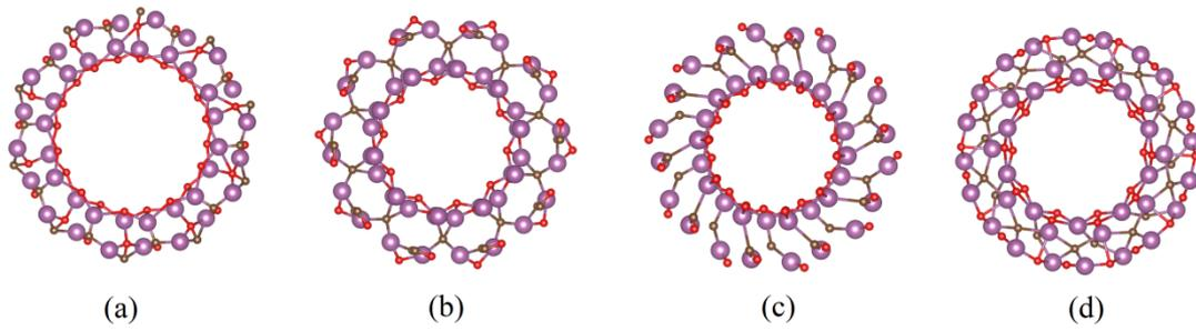
**Figure S2.** Atomic structures of (10,10) armchair  $\text{Sc}_2\text{CO}_2$  nanotubes rolled from A/ $\text{Sc}_2\text{C}$ /A, B/ $\text{Sc}_2\text{C}$ /B, and A/ $\text{Sc}_2\text{C}$ /B layers, respectively.
