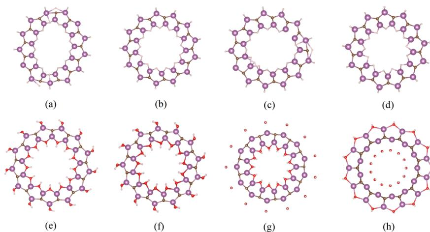
**Figure S1.** Atomic structures of (13,0) zigzag  $\text{Sc}_2\text{CH}_2$  and  $\text{Sc}_2\text{C}(\text{OH})_2$  nanotubes rolled from A/ $\text{Sc}_2\text{C}$ /A, B/ $\text{Sc}_2\text{C}$ /B, and A/ $\text{Sc}_2\text{C}$ /B layers, respectively.
