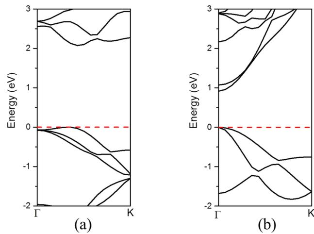
**Figure S3.** Band structures near Fermi level for the corresponding  $\text{Sc}_2\text{CH}_2$  (a) and  $\text{Sc}_2\text{C}(\text{OH})_2$  (b) monolayers along direction b, respectively.
