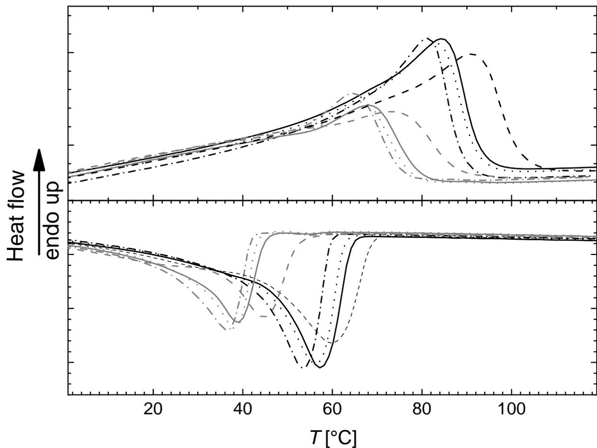
**SI Figure 2:** DSC thermograms of copolymer starting materials, PEVA20 (dashed black line), PEVA31 (dashed grey line) and crosslinked cPEVAs with different composition. cPEVA20D05 (solid black line), cPEVA20D10 (dotted black line), cPEVA20D20 (dash-dotted black line) and cPEVA31D05 (solid grey line), cPEVA31D10 (dotted grey line), and cPEVA31D20 (dash-dotted grey line) at heating and cooling rates of  $20 \text{ K}\cdot\text{min}^{-1}$ .
