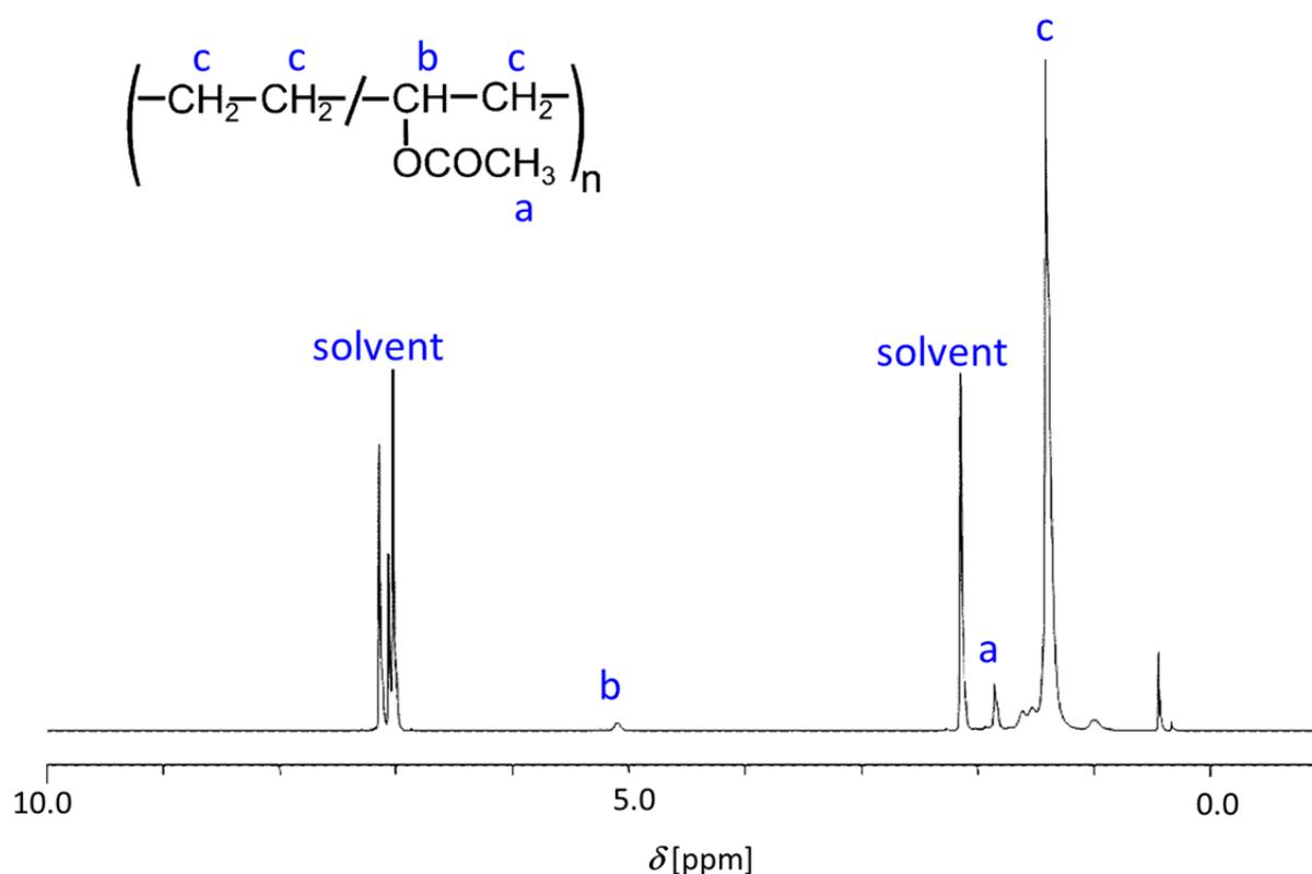
**SI Figure 1.** 500 MHz <sup>1</sup>H-NMR spectrum of cPEVA31D10 with assigned chemical shifts utilized for calculation of the average segment length of PE sequence. a:  $-\text{COOCH}_3-$  (methylene protons near the carboxyl group,  $\delta = 1.8$  ppm); b:  $-\text{CH}-$  (methylene protons near the carboxyl group,  $\delta = 5.0$  ppm); c:  $-\text{CH}_2-$  (linear methylene protons,  $\delta = 1.3$ -1.6 ppm). The solvent (toluene-d<sub>8</sub>) appears at  $\delta = 2.2$  and 7.1 ppm.
