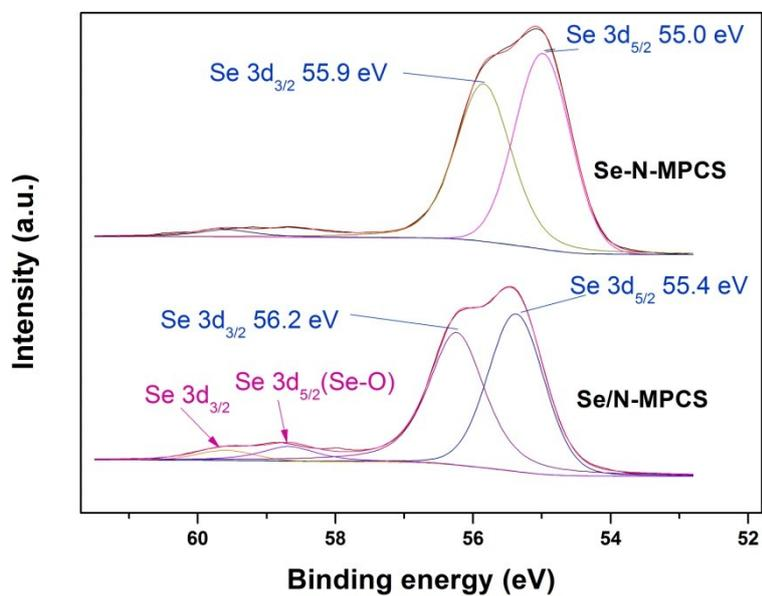
**Figure S11.** XPS spectra of Se 3d in Se/N-MPCS and Se-N-MPCS.
