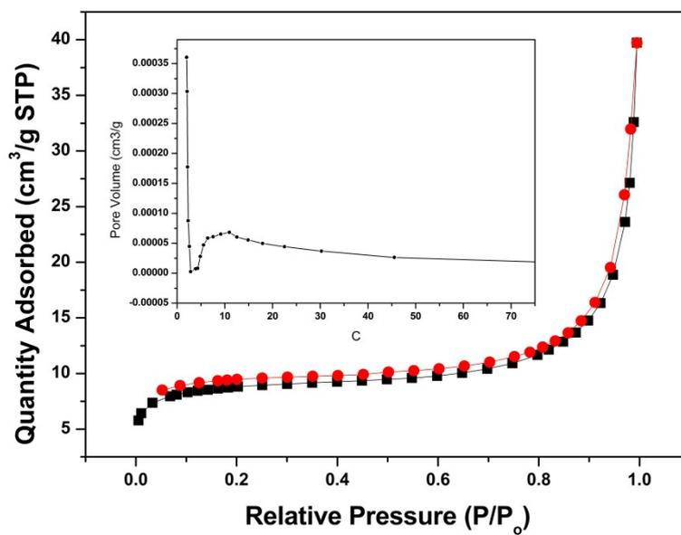
**Figure S6.** Pore size distribution of Se/N-MPCS (BET surface area = 30.1 m<sup>2</sup>/g, pore volume = 0.036 cm<sup>3</sup>/g).
