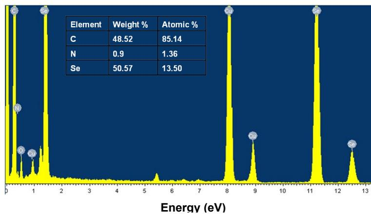
**Figure S13.** The energy dispersive X-ray spectroscopy (EDX) analysis of the Se/N-MPCS after 300 cycle.
