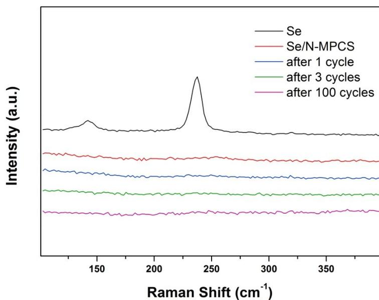
**Figure S12.** Raman spectra of selenium, Se/N-MPCS, and the Se/N-MPCS after 1 cycle, 3 cycles, and 100 cycles.
