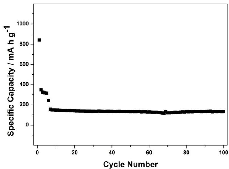
Figure S10. Cycling performance for the Se/AC at about 2 C.
