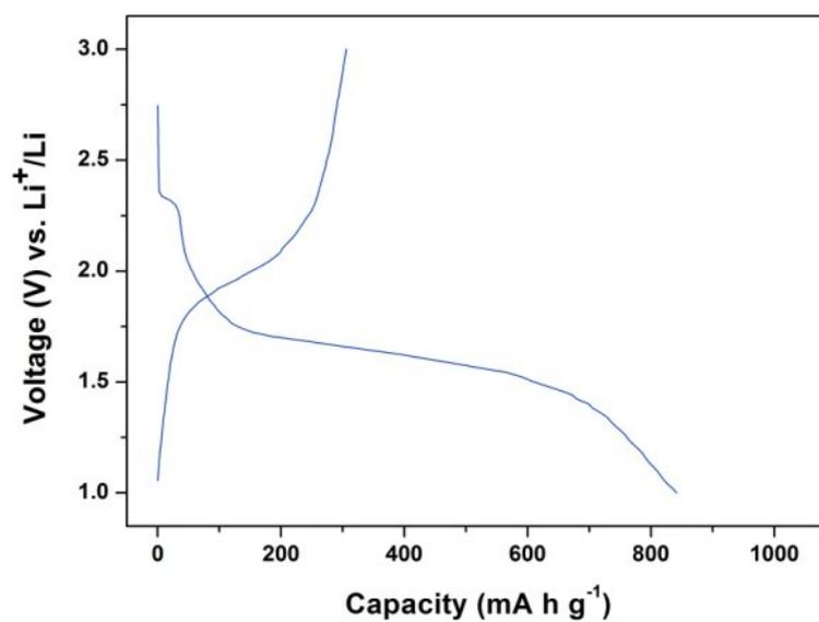
**Figure S8.** Discharge and voltage profiles for the Se/AC.
