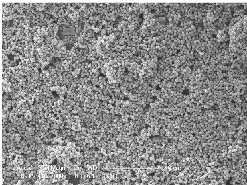
**Figure S1.** A panoramic view of the nitrogen doped microporous carbon spheres (N-MPCS).
