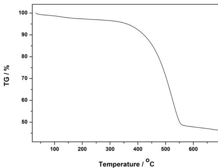
**Figure S5.** Thermogravimetric (TGA) analysis of Se/N-MPCS in nitrogen.
