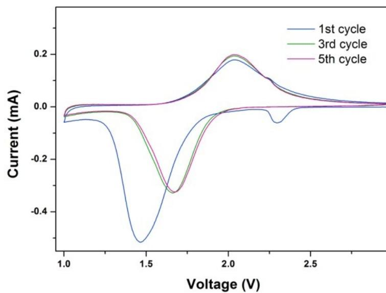
**Figure S7.** Cyclic voltammograms of Se/AC at  $0.1 \text{ mV s}^{-1}$ .
