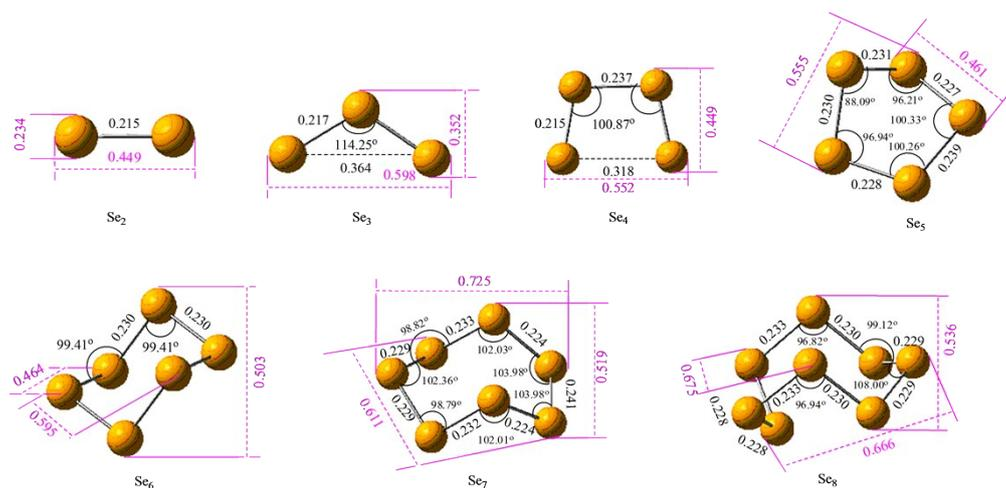
**Figure S4.** Theoretical calculation results of selenium allotropes from Se<sub>2</sub> to Se<sub>8</sub> (units of bond length: nm).
