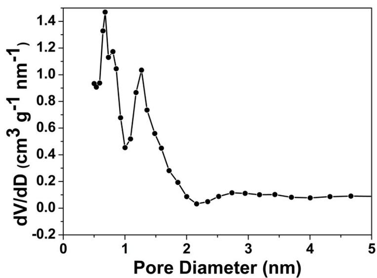
**Figure S2.** The corresponding micropore size distribution of N-MPCS.
