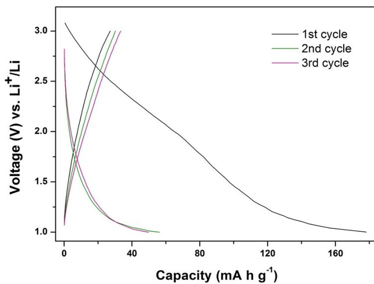
Figure S9. The discharge and charge profiles for the N-MPCS.
