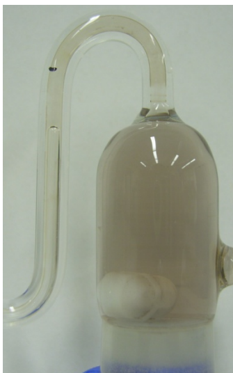
Figure S3. Photos of the water splitting solution without ZnPP after irradiation for 3 hours. [Au NPs] = 125 \mu M; [PAA 52 - b -P4VP 90 ] = 2 mg/mL; [Rh(bpy) 3 Cl 3 ] = 2 mM; [bpy] = 3 mM; [TEOA] = 0.3 M, at pH=7.5 (10 mM phosphate buffer) at 25°C.
