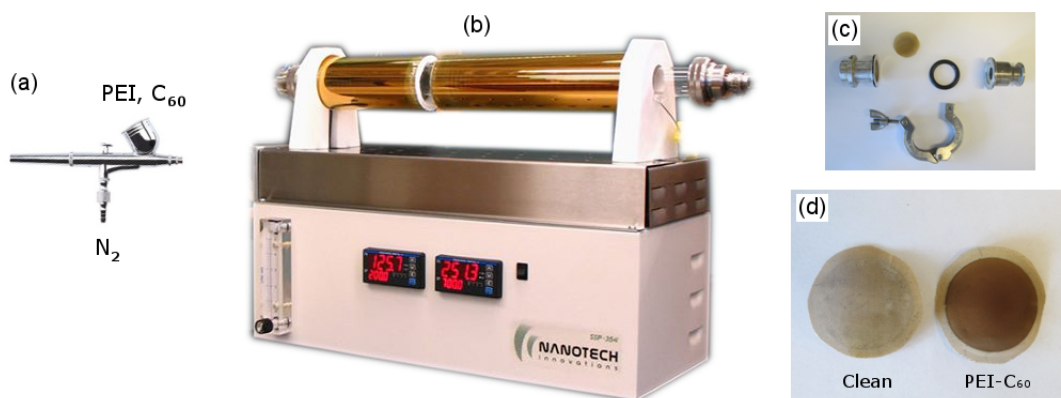
Figure S1 Components of the spray-drying equipment.
