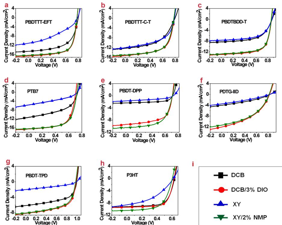
**Fig. S5** *J-V* curves based on PSCs consist of various polymer:PC<sub>71</sub>BM blends (a-h) utilizing different solvent as the processing solvent; (i) The symbols (black, red, blue, green) represented the utilized processing solvents (DCB, DCB/3% DIO, XY, XY/2% NMP), respectively.
