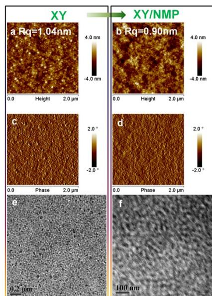
**Fig. S7** The AFM height (a, b) and phase (c, d) of PBDTT-C-T: PC<sub>71</sub>BM films made without using NMP (a, c) and with NMP (b, d) in the XY, TEM images of thin-film PBDTT-C-T:PC<sub>71</sub>BM blend cast from solutions of (e) XY only (f) 2% NMP in XY.
