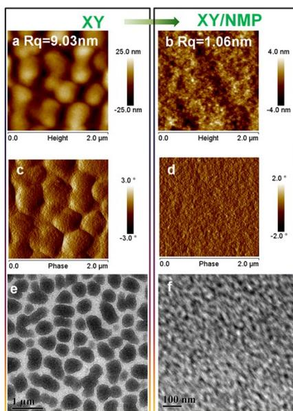
**Fig. S8** The AFM height (a, b) and phase (c, d) of PTB7: PC<sub>71</sub>BM films made without using NMP (a, c) and with NMP (b, d) in the XY, TEM images of thin-film PTB7:PC<sub>71</sub>BM blend cast from solutions of (e) XY only (f) 2% NMP in XY.
