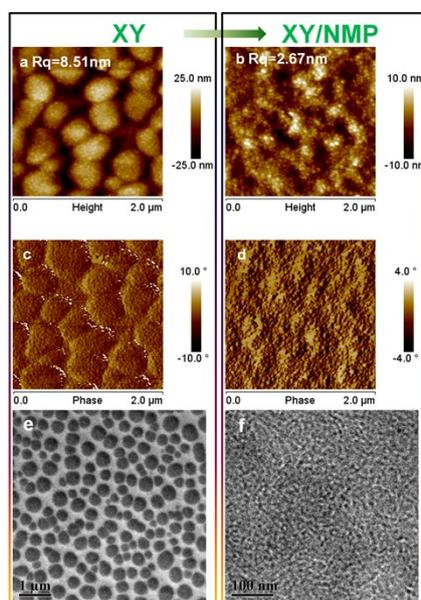
**Fig. S12** The AFM height (a, b) and phase(c, d) of PBDT-TPD: PC<sub>71</sub>BM films made without using NMP (a, c) and with NMP (b, d) in the XY, TEM images of thin-film PBDT-TPD:PC<sub>71</sub>BM blend cast from solutions of (e) XY only (f) 2% NMP in XY.
