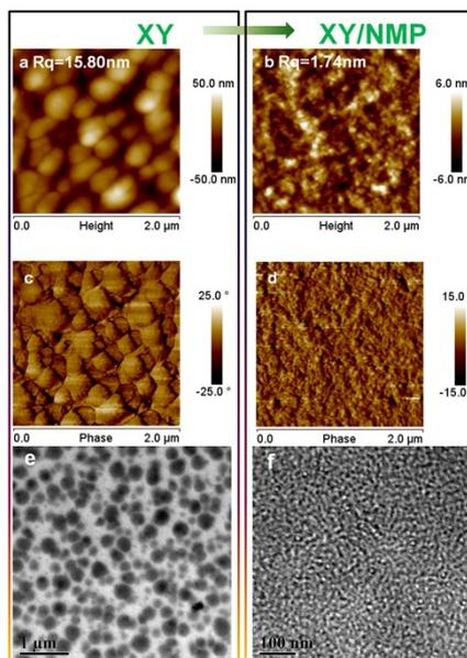
**Fig. S11.** The AFM height (a, b) and phase(c, d) of PDTG-IID: PC<sub>71</sub>BM films made without using NMP (a, c) and with NMP (b, d) in the XY, TEM images of thin-film PDTG-IID:PC<sub>71</sub>BM blend cast from solutions of (e) XY only (f) 2% NMP in XY.
