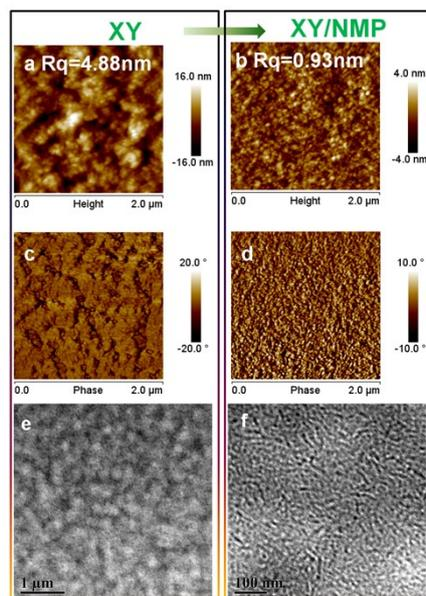
**Fig. S9** The AFM height (a, b) and phase (c, d) of PBDBTDD-T: PC<sub>71</sub>BM films made without using NMP (a, c) and with NMP (b, d) in the XY, TEM images of thin-film PBDBTDD-T:PC<sub>71</sub>BM blend cast from solutions of (e) XY only (f) 2% NMP in XY.
