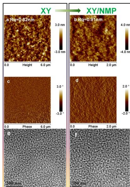
**Fig. S13** The AFM height (a, b) and phase (c, d) of P3HT: PC<sub>71</sub>BM films made without using NMP (a, c) and with NMP (b, d) in the XY, TEM images of thin-film P3HT:PC<sub>71</sub>BM blend cast from solutions of (e) XY only (f) 2% NMP in XY.
