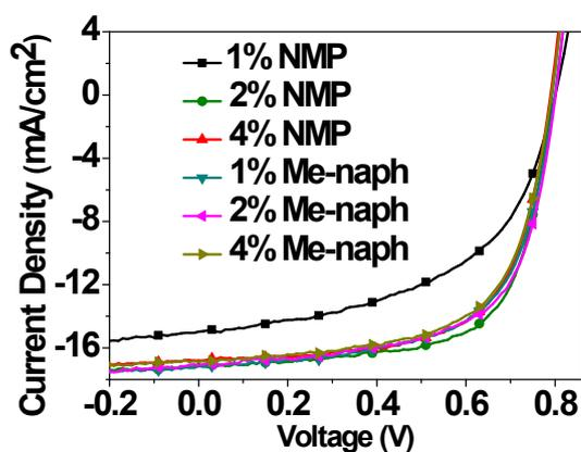
**Fig. S1.** *J-V* curves of the PSCs based on PBDT-TS1:PC<sub>71</sub>BM with different volume amount of halogen-free processing additive (NMP) and Me-naph as the processing solvent additive under the illumination of AM 1.5, 100 mW/cm<sup>2</sup>, respectively.
