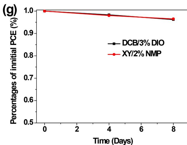
**Figure S14.** TEM images of thin-film PBBDT-TS1:PC<sub>71</sub>BM blend cast from solutions of DCB/3% DIO (a, b, c) and XY/NMP (d, e, f) every four days, respectively; (g) the corresponding PCE value plots in 8 days.
