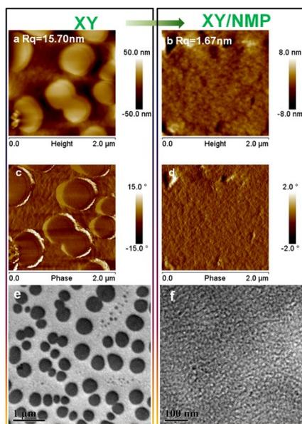
**Fig. S10** The AFM height (a, b) and phase (c, d) of PBDDT-DPP: PC<sub>71</sub>BM films made without using NMP (a, c) and with NMP (b, d) in the XY, TEM images of thin-film PBDDT-DPP:PC<sub>71</sub>BM blend cast from solutions of (e) XY only (f) 2% NMP in XY.
