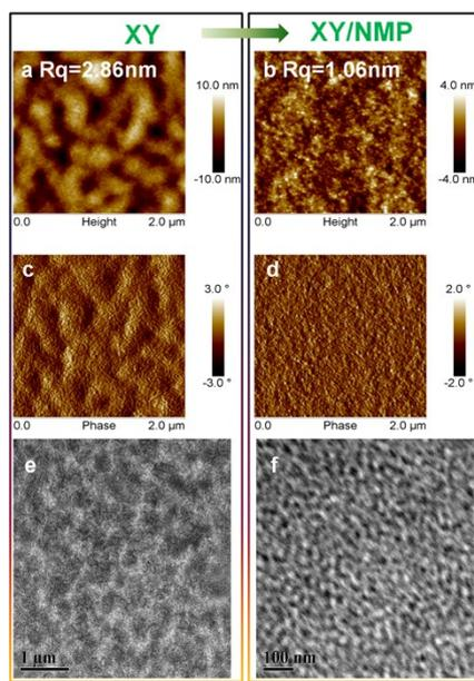
**Fig. S6** The AFM height (a, b) and phase (c, d) of PBDTT-EFT: PC<sub>71</sub>BM films made without using NMP (a, c) and with NMP (b, d) in the XY, TEM images of thin-film PBDTT-EFT:PC<sub>71</sub>BM blend cast from solutions of (e) XY only (f) 2% NMP in XY.
