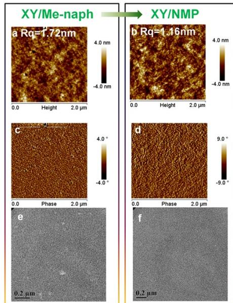
**Fig. S4** The AFM height (a, b), phase (c, d) and TEM images (e, f) of PBDT-TS1: PC<sub>71</sub>BM films cast from XY/Me-naph and XY/NMP, respectively.
