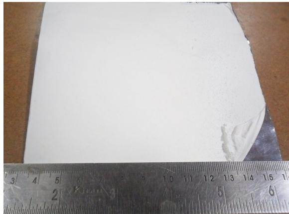
Fig. S3. Photographic image of as-spun NiAc-PVP fibrous mat
