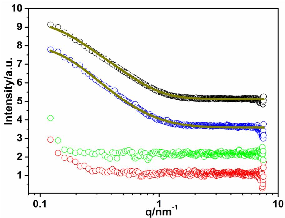
**Figure S6.** Small angle x-ray scattering (SAXS) data (open circles) of the hierarchical  $\text{Eu}_2\text{O}_3$  nanostructured powders prepared with different mass ratios of  $\text{H}_2\text{O}/\text{DMF}$ : (black) 2.5 wt%; (red) 5.0 wt%; (green) 10 wt%; (blue) 20 wt%; and shown together with simulated curves (dark yellow solid lines).
