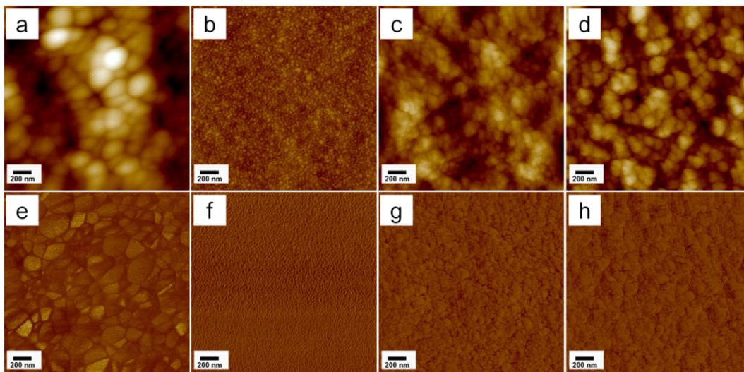
**Figure S9.** AFM height (a-d) and phase (e-h) images of pure PS-*b*-PMAA DBC films spin coated on Si substrate after solvothermal reaction for 12 hours at 170 °C with different mass ratios of H<sub>2</sub>O/DMF: (a, e) 2.5 wt%; (b, f) 5.0 wt%; (c, g) 10 wt%; (d, h) 20 wt%. Height scale: 40 nm, phase scale: 40 nm.
