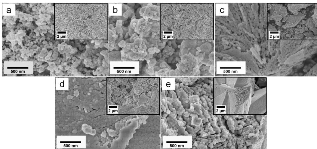
**Figure S8.** SEM images of  $\text{Eu}_2\text{O}_3$  synthesized with different mass ratios of  $\text{H}_2\text{O}/\text{DMF}$  (without  $\text{PS-}b\text{-PMAA}$ ): (a) 0; (b) 2.5 wt%; (c) 5.0 wt%; (d) 10 wt%; (e) 20 wt%, insets: low-magnification SEM images.
