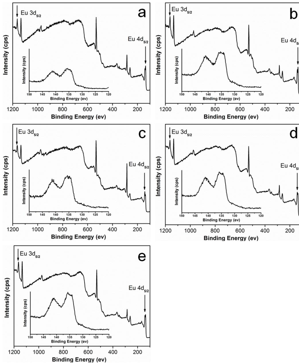
**Figure S5.** XPS profiles of the hierarchical  $\text{Eu}_2\text{O}_3$  nanostructured powders prepared with different mass ratios of  $\text{H}_2\text{O}/\text{DMF}$ : (a) 0; (b) 2.5wt%; (c) 5.0 wt%; (d) 10 wt%; (e) 20 wt%. Inset: detailed XPS of the 4d electron of  $\text{Eu}^{3+}$ .
