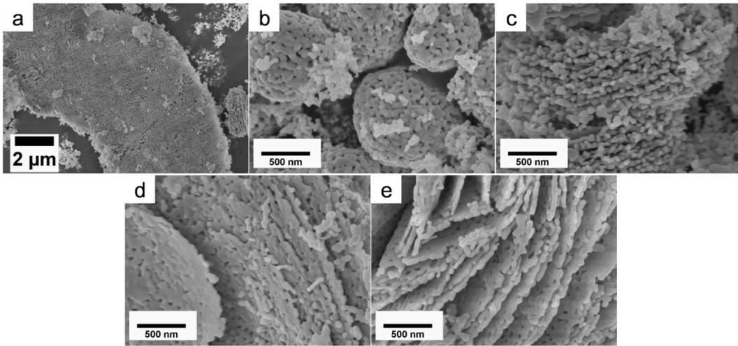
**Figure S1.** SEM images of the hierarchical Eu<sub>2</sub>O<sub>3</sub> nanostructured powders prepared with different mass ratios of H<sub>2</sub>O/DMF: (a) 0; (b) 2.5 wt%; (c) 5.0 wt%; (d) 10 wt%; (e) 20 wt%.
