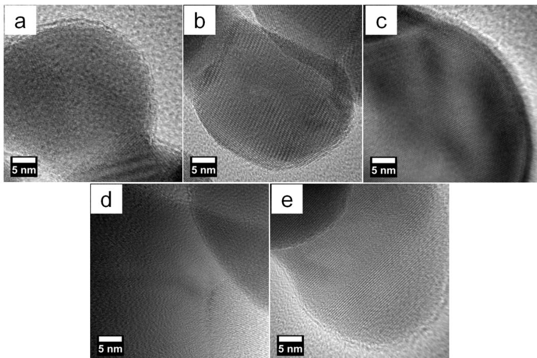
**Figure S3.** HRTEM images of the hierarchical  $\text{Eu}_2\text{O}_3$  nanostructured powders prepared with different mass ratios of  $\text{H}_2\text{O}/\text{DMF}$ : (a) 0; (b) 2.5 wt%; (c) 5.0 wt%; (d) 10 wt%; (e) 20 wt%.
