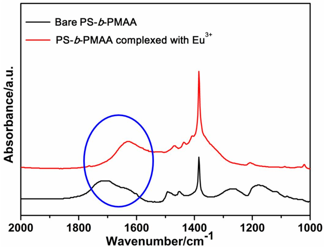
**Figure S2.** FT-IR profiles of pure PS-*b*-PMAA DBC (black) and PS-*b*-PMAA DBC complexed with Europium Nitrate (red). The marked regions indicate the red shift of the carbonyl stretching band (1716 cm<sup>-1</sup> vs. 1648 cm<sup>-1</sup>).
