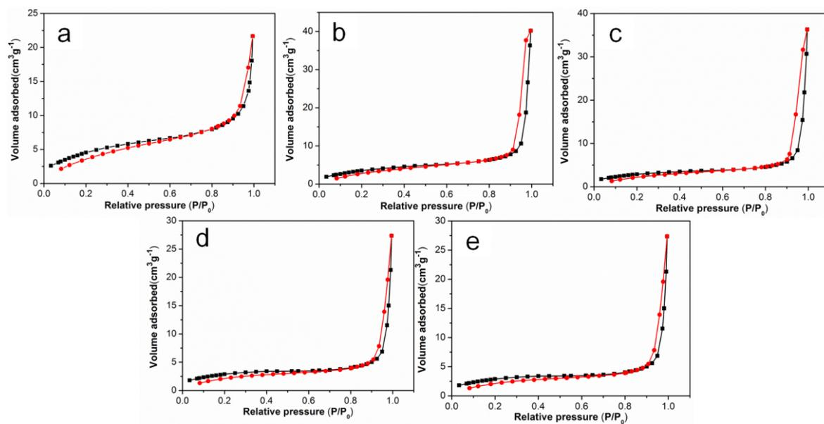
**Figure S7.** Nitrogen physisorption isotherms of the micro-nano  $\text{Eu}_2\text{O}_3$  powder prepared with different mass ratios of  $\text{H}_2\text{O}/\text{DMF}$ : (a) 0; (b) 2.5 wt%; (c) 5.0 wt%; (d) 10 wt%; (e) 20 wt%.
