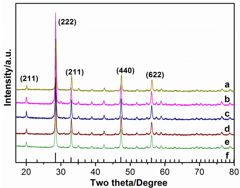
**Figure S4.** XRD patterns of the hierarchical Eu<sub>2</sub>O<sub>3</sub> nanostructured powders prepared with different mass ratios of H<sub>2</sub>O/DMF: (a) 0; (b) 2.5wt%; (c) 5.0 wt%; (d) 10 wt%; (e) 20 wt%; (f) standard XRD pattern of Eu<sub>2</sub>O<sub>3</sub>.
