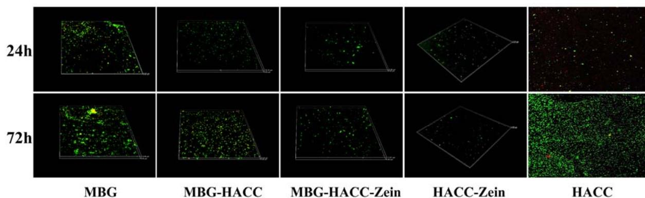
Supplemental Fig. 2 Projected top views of antibacterial efficacy of different scaffolds against *Escherichia coli* at 24h and 72h obtained using confocal laser scanning microscopy (CLSM) after staining with the Baclight dead/live stain. Bacteria were stained with green fluorescent SYTO 9 and red fluorescent propidium iodide, which causes live cells to appear green and dead cells to appear red under CLSM. Magnification,  $\times 400$ .
