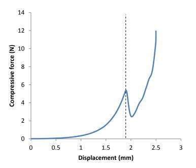
Example compression test, showing the point at which alginate matrices fracture
