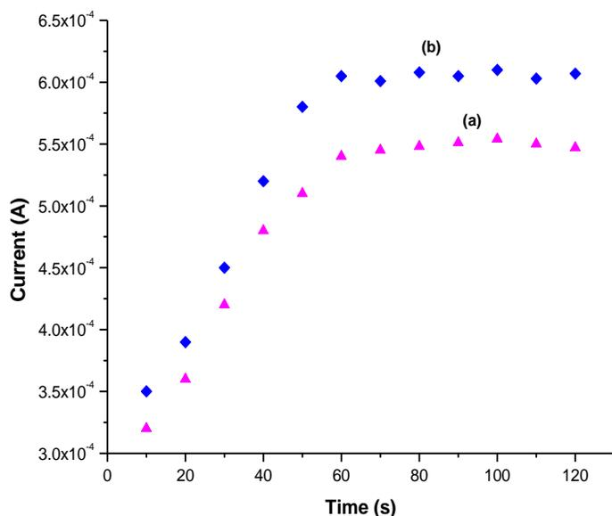
**Fig. S4** Response time curve showing variation of peak current with time (a) ChOx/Fe<sub>3</sub>O<sub>4</sub>@ C film/ITO bioelectrode, and; (b) ChOx/ $\alpha$ -Fe<sub>2</sub>O<sub>3</sub> film/ITO bioelectrode.
