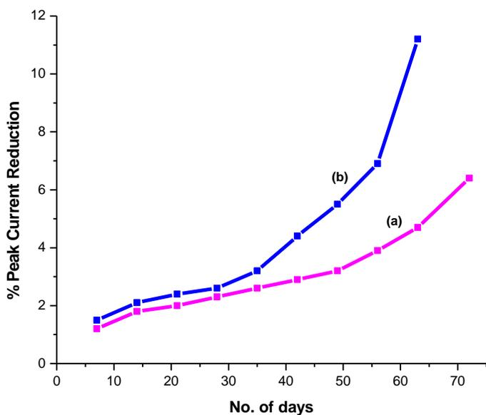
**Fig. S2** Shelf life curves showing % reduction in peak current with time (a) ChOx/Fe<sub>3</sub>O<sub>4</sub>@ C film/ITO bioelectrode, and; (b) ChOx/ $\alpha$ -Fe<sub>2</sub>O<sub>3</sub> film/ITO bioelectrode.
