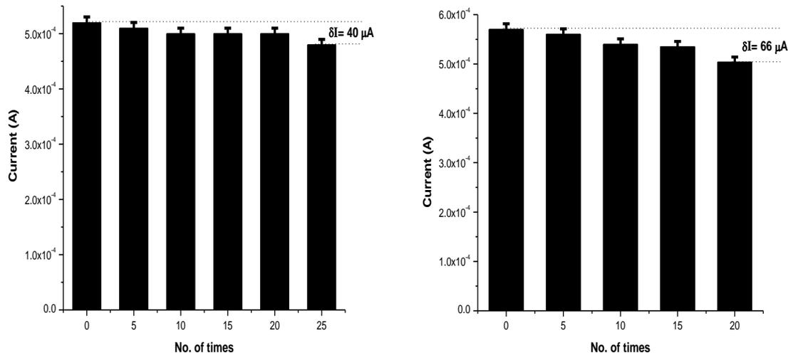
**Fig. S3** Reproducibility curve showing reduction in peak current with no. of usage times (a) ChOx/Fe<sub>3</sub>O<sub>4</sub>@ C film/ITO bioelectrode, and; (b) ChOx/ $\alpha$ -Fe<sub>2</sub>O<sub>3</sub> film/ITO bioelectrode.
