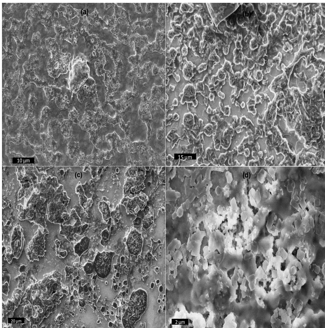
**Fig. S1** SEM micrographs after ChOx immobilization onto: (a)  $\alpha$ - $\text{Fe}_2\text{O}_3$  NPs film obtained from  $\text{Fe}_3\text{O}_4$  NPs; (b)  $\alpha$ - $\text{Fe}_2\text{O}_3$  NPs film obtained from  $\text{Fe}_3\text{O}_4$  NPs (autoclaved); (c) film of  $\text{Fe}_3\text{O}_4@ \text{C}$  NPs; (d) film of  $\text{Fe}_3\text{O}_4@ \text{SiO}_2$  NPs.
