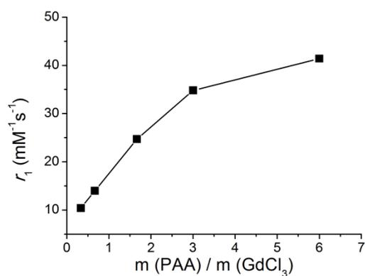
Fig. S7 The  $r_1$  relaxivity of PAA-coated gadolinium hydrated carbonate nanoparticles synthesized in the presence of different amounts of PAA.  $r_1$  was plotted as a function of m(PAA)/m(GdCl<sub>3</sub>). The nanoparticles were synthesized using the same method except for the amount of PAA added.
