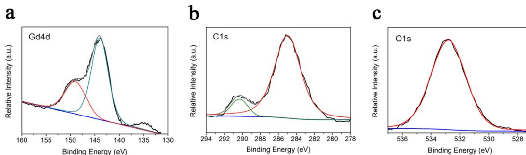
Fig. S5 XPS spectra for naked gadolinium hydrated carbonate nanoparticles: (a) Gd 4d, (b) C 1s, and (c) O 1s.
