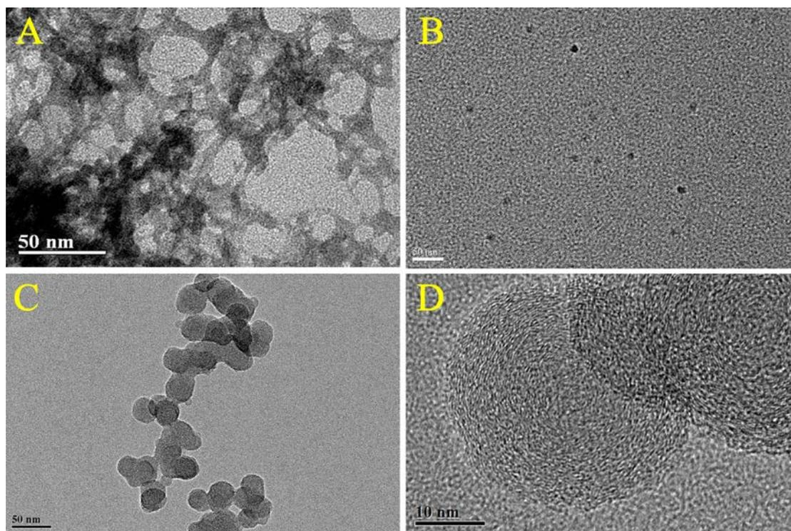
Fig. S3 TEM image of gadolinium hydrated carbonate nanoparticles synthesized (A) without PAA, (B) with 0.2g PAA, (C) and (D) with 0.1g PAA.
