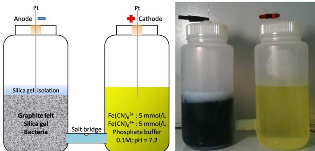
ESI-5: Scheme (left) and picture (right) of a H-type microbial fuel cell realized with gelified felt. Anode volume is 240 cm<sup>3</sup>.
