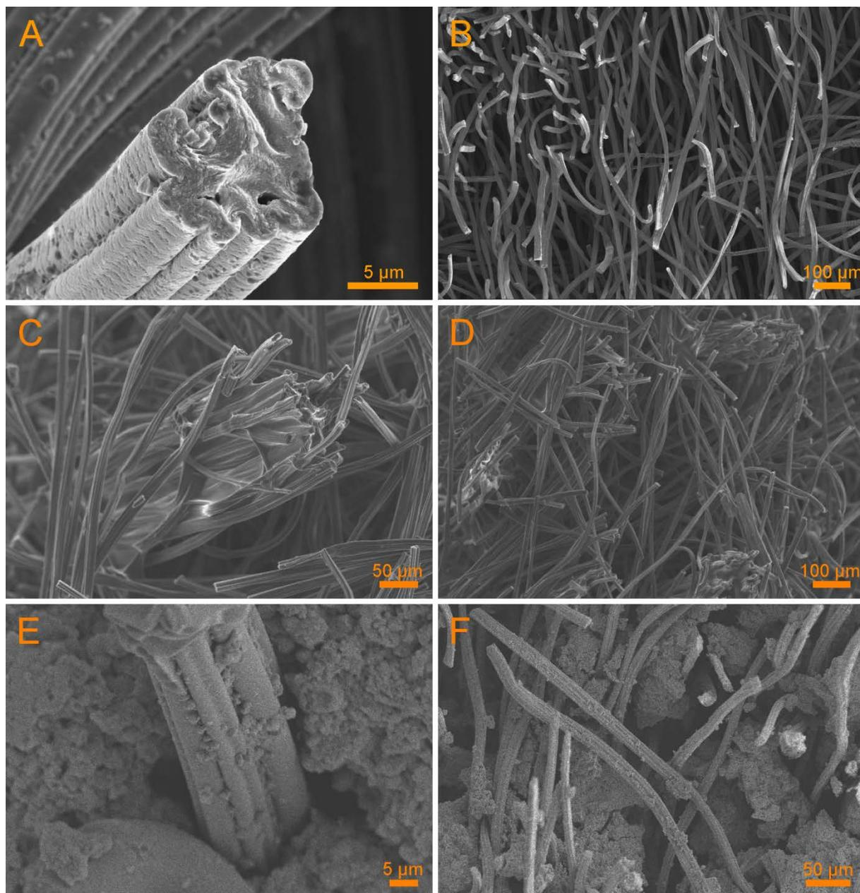
ESI-1: SEM views of (A,B) untreated, (C,D) alginate-treated and (E,F) silicified graphite felt. A: close view of a graphite fiber. B: general view of the untreated felt. C: fibers bundled together by the alginate deposit. A thinner deposit can be seen on neighbouring non-aggregated fibers. D: general view of the alginate-treated felt. E: fiber embedded in the silica matrix. F: silicified graphite felt.
