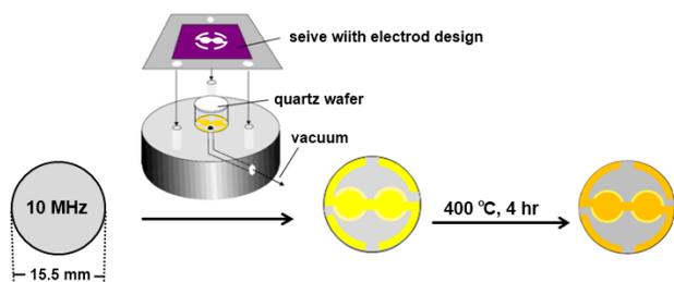
Fig.S1 Screen printing process of dual gold quartz crystal microbalance.
