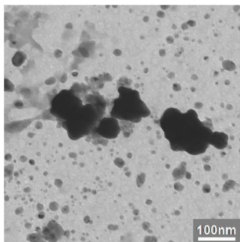
**Figure S3.** TEM image of the product prepared without pre-adsorption of  $\text{Au}^{3+}$  ions before the addition of ascorbic acid reductant into the reaction mixture.
