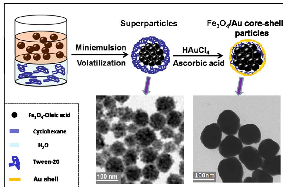
**Scheme S1** Schematic presentation of the synthetic procedure for the  $\text{Fe}_3\text{O}_4/\text{Au}$  core-shell particles.
