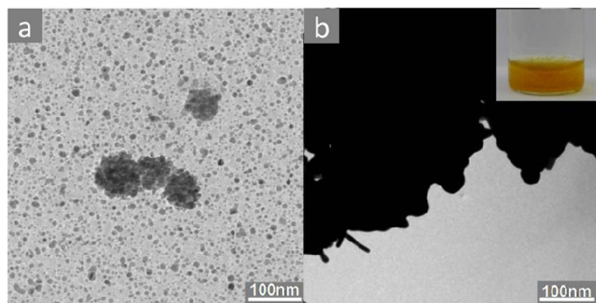
**Figure S4.** TEM images of the products prepared from (a) sodium dodecylsulfate (SDS) modified  $\text{Fe}_3\text{O}_4$  SPs and (b) dodecyl trimethyl ammonium bromide (DTAB) modified  $\text{Fe}_3\text{O}_4$  SPs. Insert of (b) shows the photograph of the dispersion of the DTAB modified  $\text{Fe}_3\text{O}_4$  SPs after addition of  $\text{HAuCl}_4$ .
