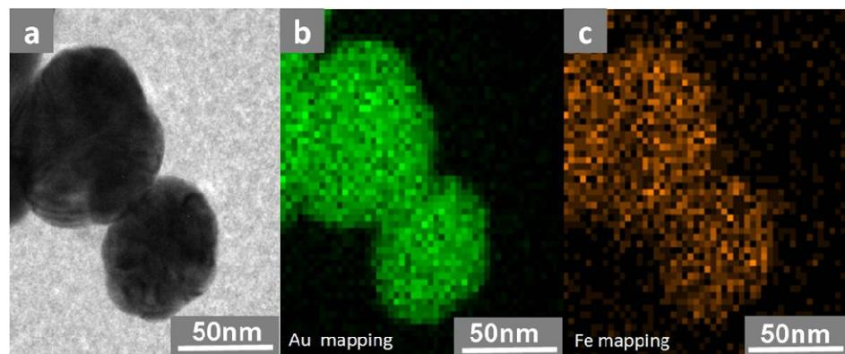
**Figure S1.** (a) High angle annular dark field scanning TEM (HAADF-STEM) image and (b, c) HAADF-STEM energy dispersive spectrometer (HAADF-STEM-EDS) mapping images of the  $\text{Fe}_3\text{O}_4/\text{Au}$  core-shell particles prepared with 8.4 mM.  $\text{HAuCl}_4$ .
