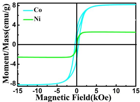
Figure S3: Magnetization loops of Co and Ni-wings.
