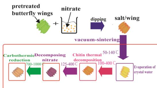
Scheme S1: Scheme of the procedure used to synthesize Fe-wing with the microstructure of butterfly wing scales.
