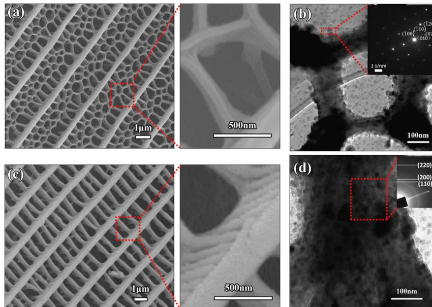
Figure S1: (a,b) SEM images of original PP fore-wing and HG wing respectively; (b,d) TEM images of Fe-PP fore-wing and Fe-HG wing respectively, the inset in (b,d) are the selected-area electron diffraction (SAED) patterns.
