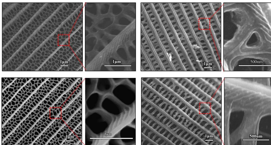
Figure S4: (a1,a2) Surface morphology of as-synthesized Co-wings, (b1,b2) Surface morphology of as-synthesized Ni-wings.
