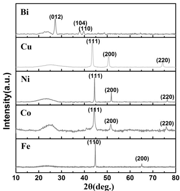
Figure S2: XRD pattern of the Fe-wing in air at room temperature for one month; and XRD patterns of Co, Ni, Cu and Bi-wings calcined in vacuum at 800°C.
