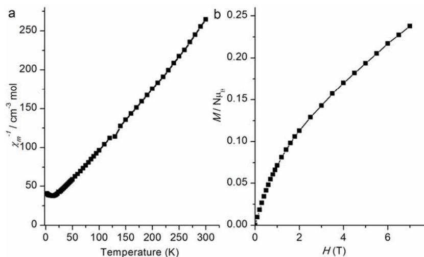
**Figure S4.** Magnetic properties of HISS. a)  $\chi^{-1}$ -T and b) M-H curves.
