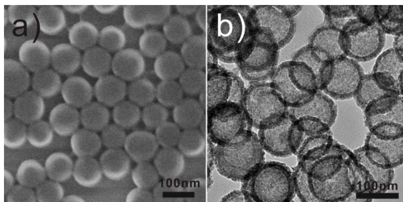
**Figure S1.** a) SEM image of the silica template and b) TEM image of the as-prepared hollow iron silicate nanoparticles
