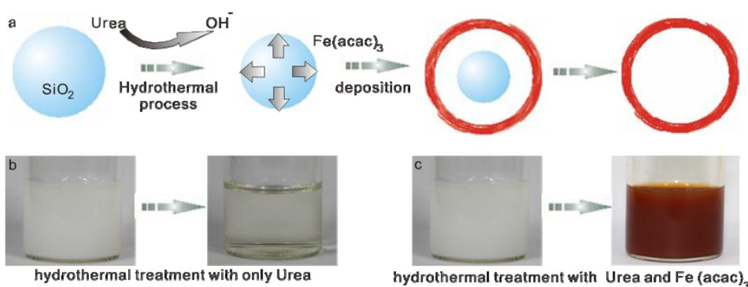
**Scheme S1.** a) Mechanism of HISS preparation, b) after hydrothermal treatment with urea, SiO<sub>2</sub> template dissolved, c) in the presence of iron acetylacetonate, HISS could be synthesized.
