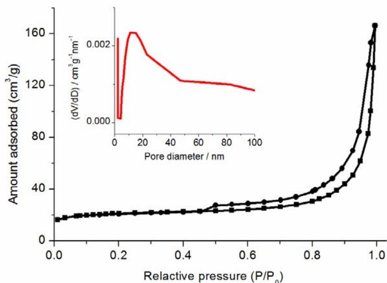
**Figure S2.** N<sub>2</sub> adsorption/desorption isotherm and the pore size distribution (inset) of HISS.
