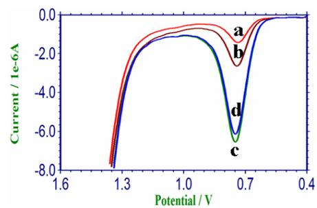
**Fig. S3** Representative DPV in B-R solution with  $2 \times 10^{-4}$  mol/L guanine recorded at GNO-SPAN with different ultrasonic time s (a) 10 min, (b) 20 min, (c) 30 min, (d) 40 min.
