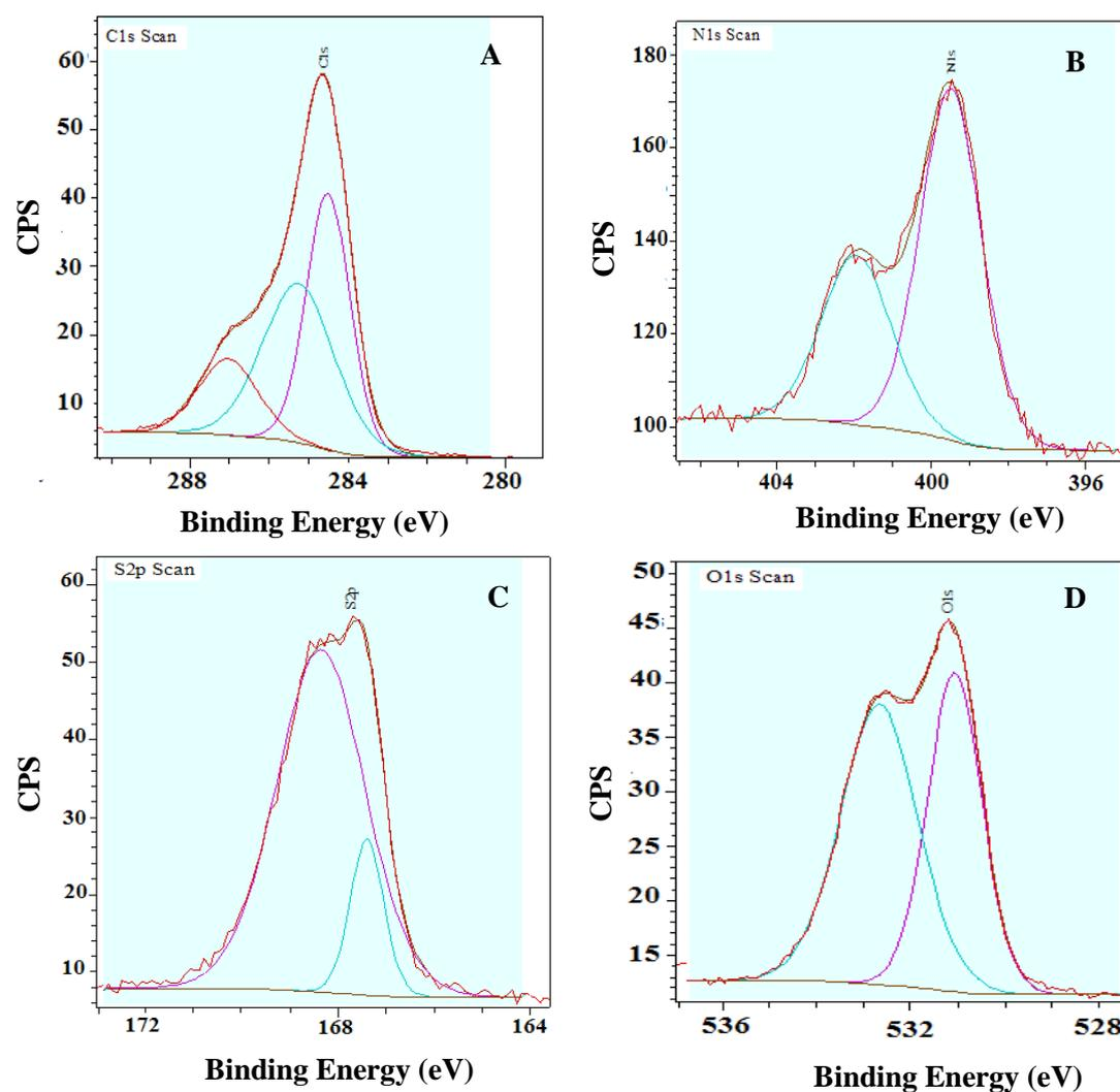
Fig. S1 The C 1s(A), N 1s(B), O 1s (C) and S 2p (D) XPS spectrum of GNO-SPAN. Note: count per second (CPS)
