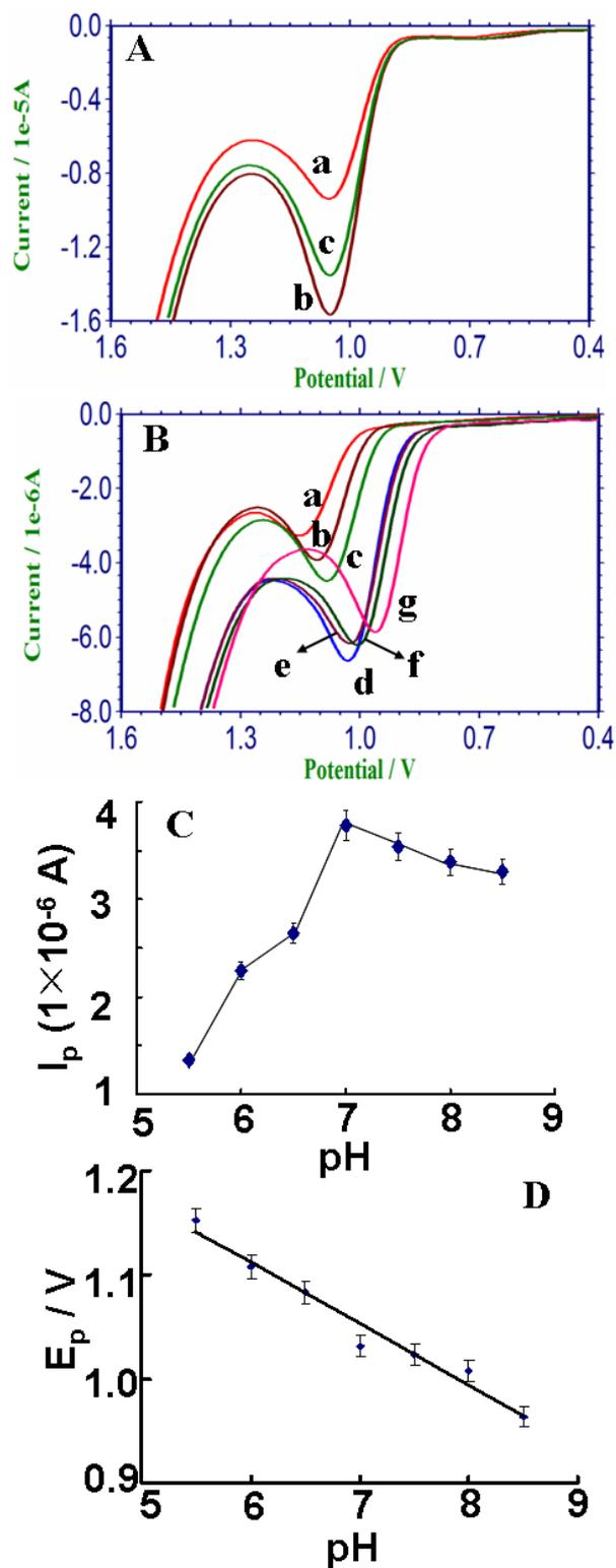
**Fig. S2** (A) Representative DPV of  $2 \times 10^{-4}$  mol/L adenine in ABS (a), B-R (b) and PBS (c) buffer solutions. (B), (C), (D) The effect of pH on the electrooxidation of  $5.0 \times 10^{-5}$  mol/L adenine. (a)–(g) 5.5, 6.0, 6.5, 7.0, 7.5, 8.0 and 8.5. *Note:* Each point is the mean of three measurements, and the error bars correspond to the standard deviation.
