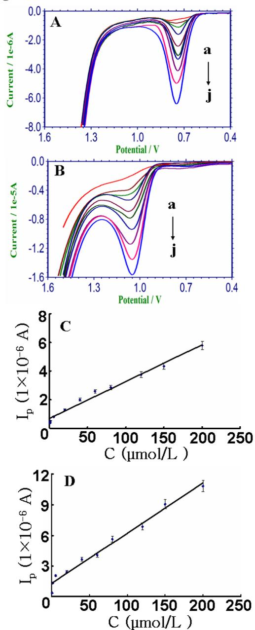
**Fig. S4** Representative DPV of guanine (A) and adenine (B) (from a to j: 0.5, 1, 5, 20, 40, 60, 80, 120, 150 and 200 μmol/L) at GNO-SPAN/CPE in B-R. Calibration curves of the oxidation peak current versus different concentration of guanine (C) and adenine (D), respectively. *Note:* Each point is the mean of three measurements, and the error bars correspond to the standard deviation.
