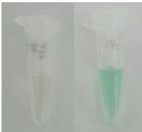
Figure S4. Color response of DNAzyme system in the absence (left, colorless) or presence (right, blue-green) of complex 1 .
