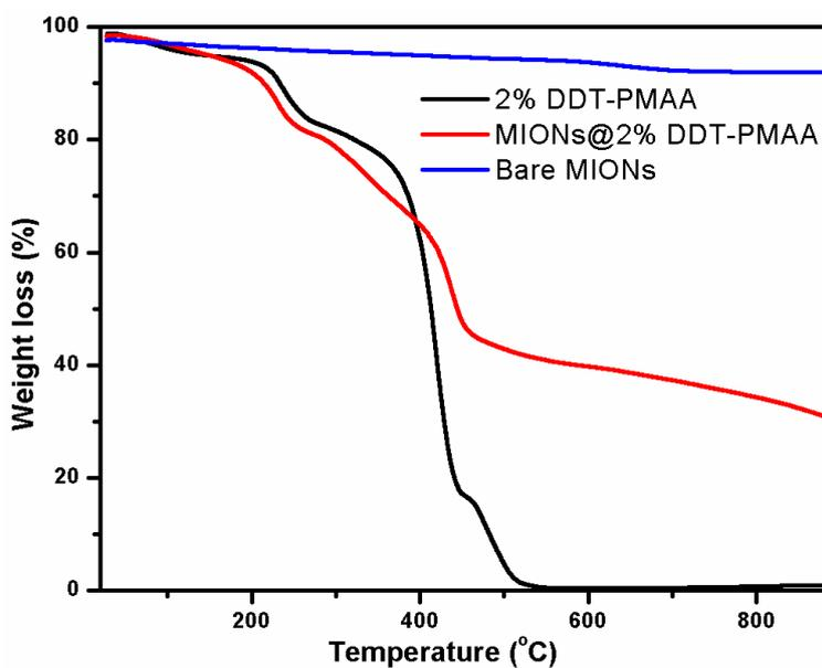
Fig. S9 TGA curves of 2%DDT-PMAA, MIONs with 2%DDT-PMAA (1.5 mM) and bare MIONs.
