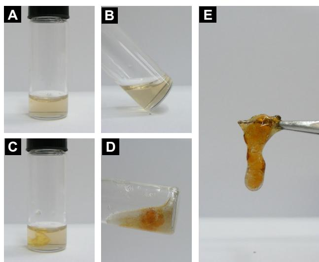
**Supplementary Figure 1.** Macroscopic images of DOPA-gelatin (A, B) and DOPA- $\text{Fe}^{3+}$  gelatin hydrogels (C, D, E). The addition of 10 mM  $\text{FeCl}_3$  solution induced a rapid hydrogel formation of DOPA-gelatin within seconds (C, D). (E) A DOPA- $\text{Fe}^{3+}$  gelatin hydrogel formed after gentle agitation for 1 h.
