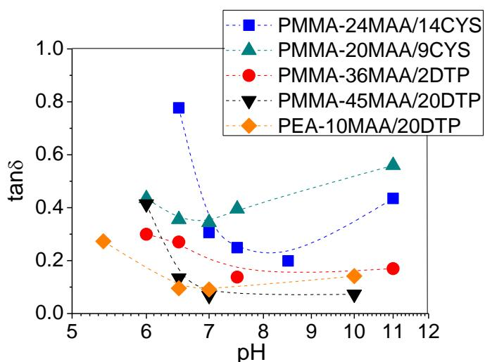
**Fig. S7.** Variation of  $\tan\delta$  with pH for PMMA-MAA and PEA-MAA-based crosslinked particles
