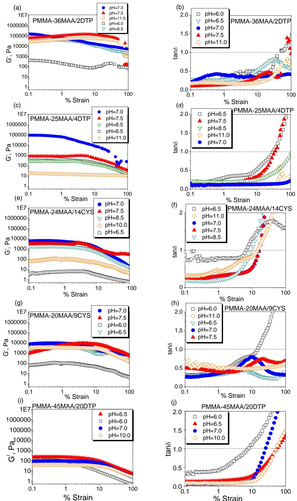
**Fig. S8.** The variation of  $G'$  and  $\tan\delta$  with the percentage strain for various PMMA-MAA-based crosslinked particle gels.
