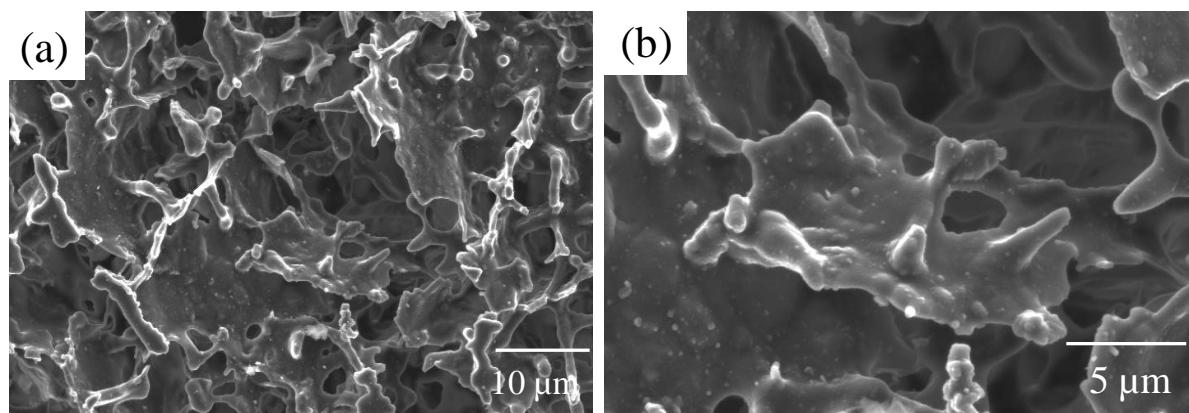
**Fig. S6.** SEM images of freeze-dried PMMA-25MAA/4DTP gels formed at pH 7.0
