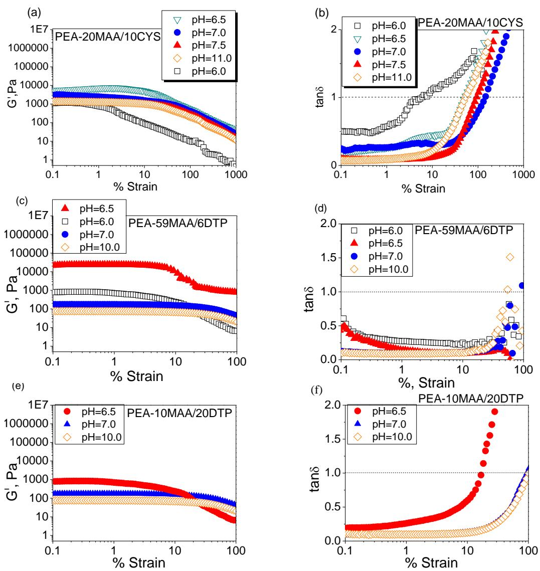
**Fig. S9.** The variation of (a)  $G'$  and (b)  $\tan\delta$  with the percentage strain for PEA-MAA-based crosslinked particle gels.
