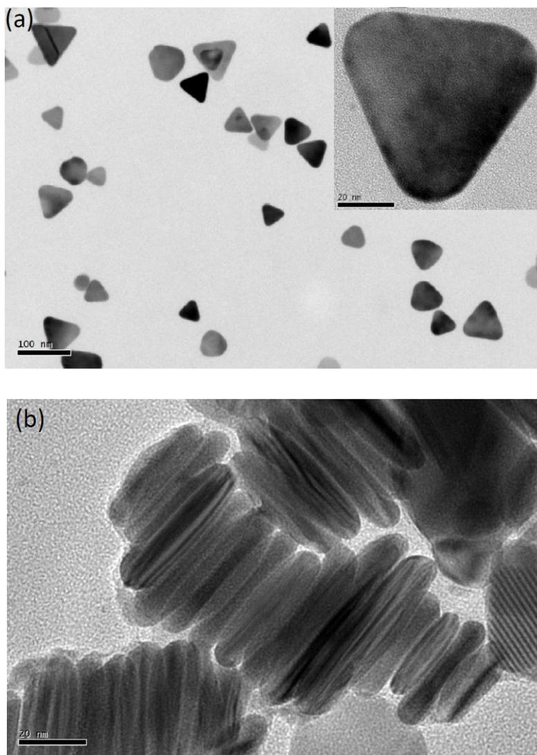
**Figure S6** TEM images of Ag triangular plates: (a) front view, and (b) side view.
