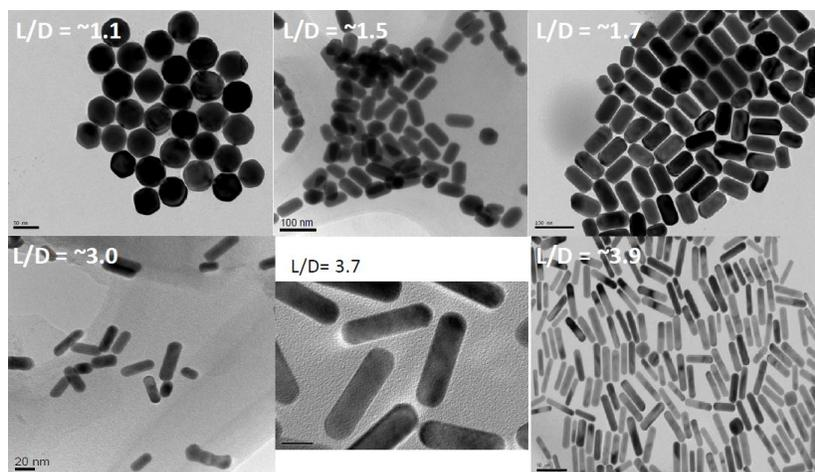
**Figure S9** TEM images of single crystalline Au NRs with different aspect ratios (L/D) as labeled in the figure.
