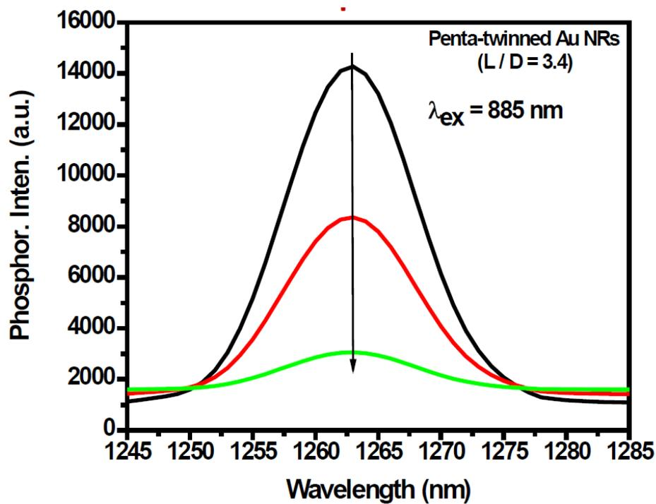
**Figure S2** Quenching of singlet O<sub>2</sub> phosphorescence emission after purging argon into the solution for 5 and 10 minutes. Singlet O<sub>2</sub> was formed via sensitization of penta-twinned Au NRs (L/D=3.4, λ<sub>ex</sub>=885 nm).
