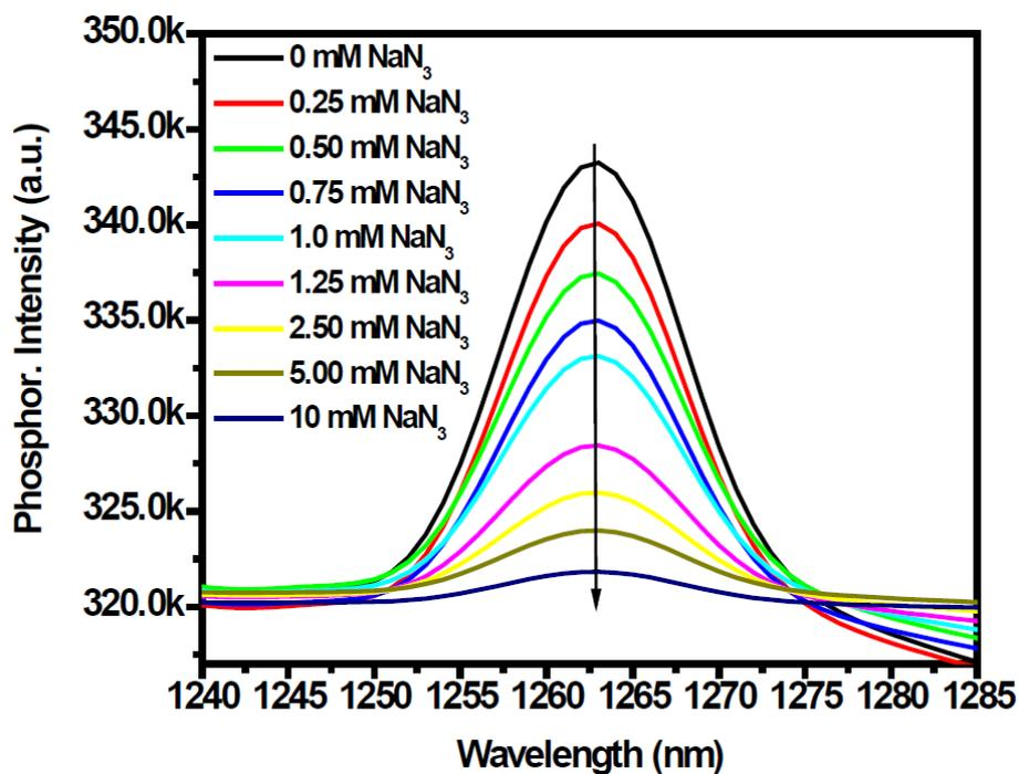
**Figure S1** Quenching of singlet O<sub>2</sub> phosphorescence by different concentrations of sodium azide. Singlet O<sub>2</sub> was formed via sensitization of penta-twinned Au NRs (L/D=3.4,  $\lambda_{ex}$ = 885 nm). The residual fraction of unquenched singlet O<sub>2</sub> phosphorescence is of ~6.5%.
