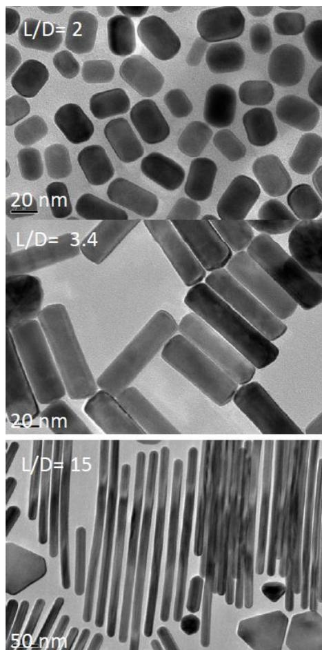
**Figure S8** TEM images of penta-twinned Au NRs with different aspect ratios (L/D) as labeled in the figure.
