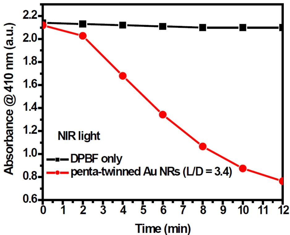
**Figure S3** Time course absorption of DPBF containing solutions of penta-twinned Au NRs (L/D = 3.4) under the photoirradiation of NIR light for 12 min. 300 W halogen lamp equipped with a band pass filter of 750 -1380 nm to cut off the UV and visible lights. The light intensity measured at 850 – 950 nm wavelength range was  $\sim 300 \text{ mW} / \text{cm}^2$ .
