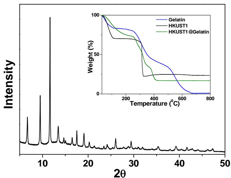
**Figure S10.** PXRD characterisation data of HKUST-1@gelatin composites; the inset shows TGA data and indicates a MOF content of 70% for the composite.
