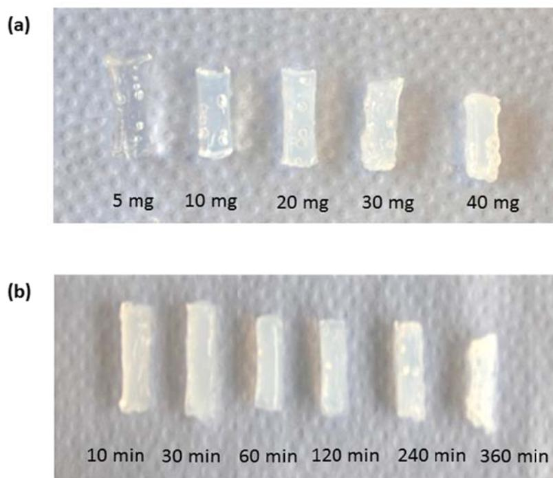
**Figure S9.** Digital photographs of (a) Zn(II)@gelatin precursor pellets of varying Zn contents following soaking in ethanolic 2-MeIm solution for 24 hrs. b) Zn(II)@gelatin precursor pellets containing 40 mg of Zn following soaking in ethanolic 2-MeIm solution for varying periods of time.
