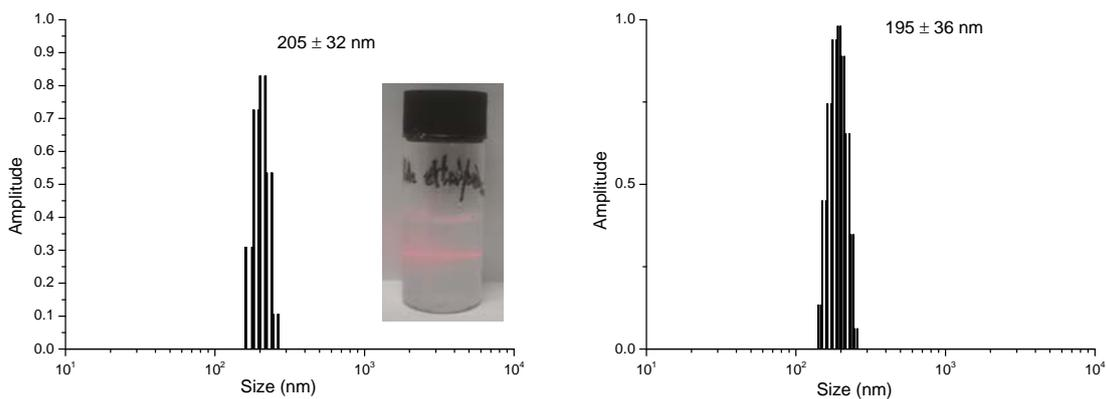
**Figure S4.** DLS data of a redispersed ZIF-8@gelatin composite after reaction for 24 hrs (left) and after standing for 2 months (right). The inset is a demonstration of the Tyndall effect by the (re)dispersed composite colloids.
