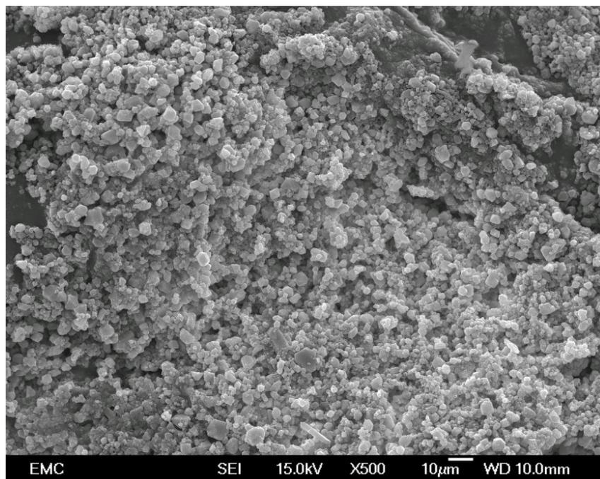
**Figure S15.** SEM image of HKUST-1 prepared solvothermally at 120 °C in 50/50 EtOH/H<sub>2</sub>O in the presence of 0.1% gelatin, revealing a mesostructured aggregate of microparticles.
