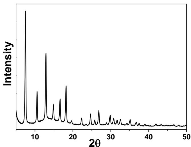
**Figure S7.** PXRD pattern of ZIF-8 recovered from ZIF-8@gelatin composites after removal of the biopolymer by repeated washing in hot water.
