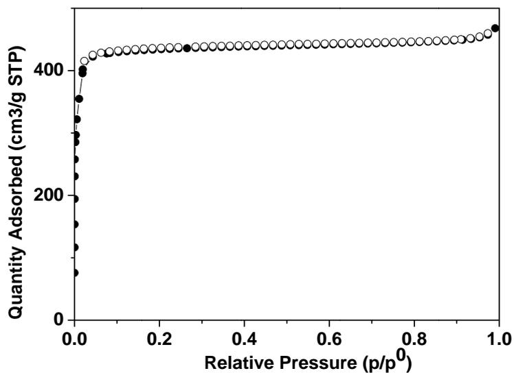
**Figure S13.** N<sub>2</sub> isotherm data for ZIF-8 crystals prepared in the presence of 0.1 wt% gelatin. The apparent BET surface area is 1281 m<sup>2</sup>/g which is only slightly lower than previous reports for ZIF-8 nanoparticles.
