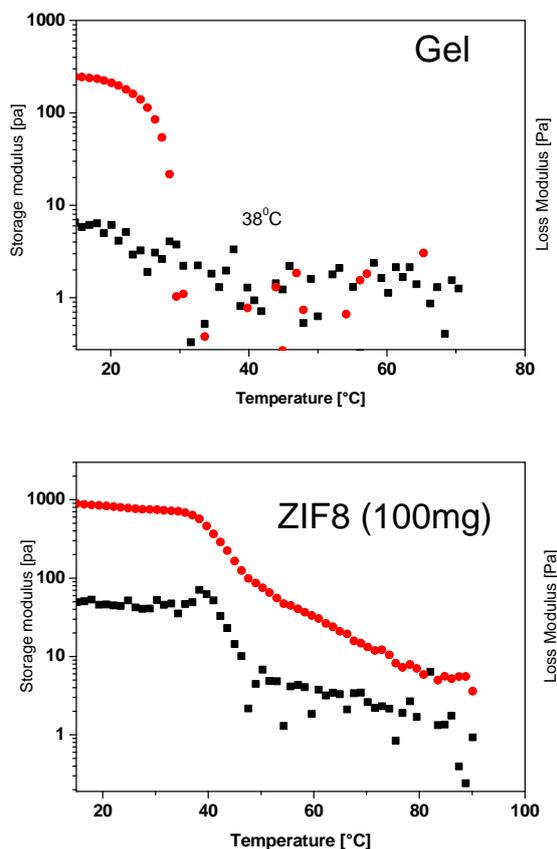
**Figure S3.** The oscillatory viscoelastic temperature ramp curve of pure 5 wt% gelatin gel and ZIF-8@gelatin composite (prepared from a starting amount of 100mg zinc nitrate hexahydrate) at a constant frequency of 1 Hz (red symbol– storage modulus, black symbol - loss modulus).
