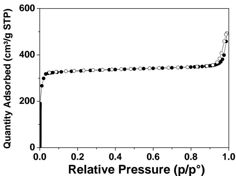
**Figure S8.** N<sub>2</sub> isotherm data for ZIF-8 recovered from ZIF-8@gelatin composites after removal of the biopolymer by repeated washing in hot water. The apparent BET surface area is 1350 m<sup>2</sup>/g, and the upturn at high relative pressure is consistent with the small particle size previously observed by SEM.
