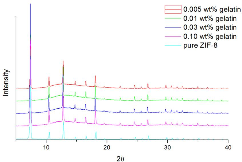
**Figure S12.** PXRD data of ZIF-8 prepared in the presence of small amounts of gelatin added as a soluble macromolecular additive. See also table S3.
