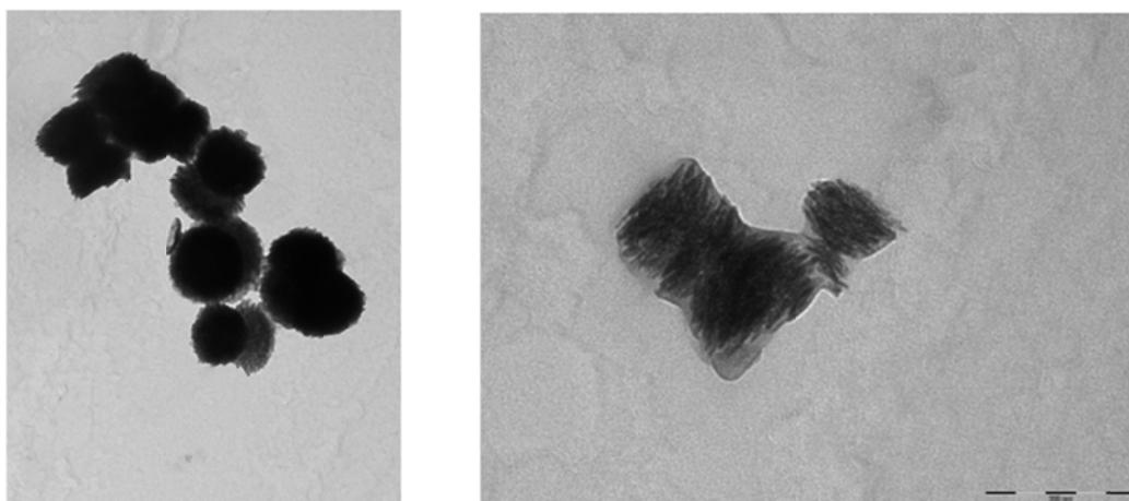
**Figure S6.** TEM images of ZIF-8@gelatin composites, prepared by pipetting 2-month old aqueous redispersions onto the grids.
