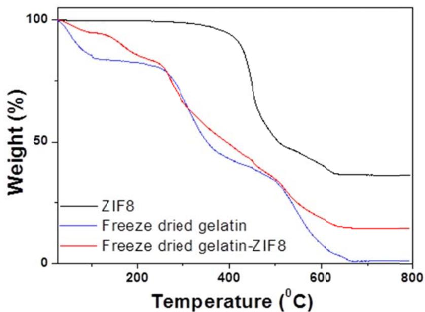
**Figure S2.** Thermogravimetric data of ZIF-8@gelatin composites compared to the individual components.
