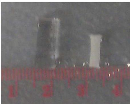
**Figure S1.** Digital photographs of a 5 wt% pure gelatin hydrogel pellet (left) and after soaking in EtOH (right). The shrinkage occurs due to partial gelatin insolubility in alcohol, and demonstrates that this does not occur due to the presence of ZIF-8.
