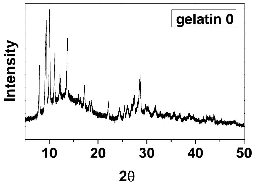
**Figure S11.** PXRD data of the product formed by the direct reaction between  $\text{Cu}(\text{OAc})_2$  and  $\text{Na}_3\text{BTC}$  in water in the absence of any gelatin. It is clear that no HKUST-1 formation has occurred, and the product is likely a mixture of the competing phases and other impurities.
