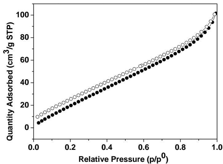
**Figure S5.** Nitrogen adsorption isotherm of ZIF-8@gelatin composite following redispersion and freeze-drying. The isotherm reveals no microporosity, consistent with the ZIF-8 particles being wholly embedded within the gelatin matrix.
