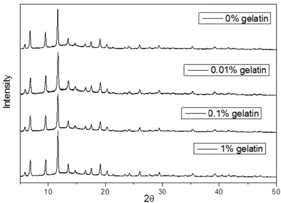
**Figure S14.** PXRD patterns of HKUST-1 prepared solvothermally at 120 °C in 50/50 EtOH/H<sub>2</sub>O in the presence of gelatin as indicated.
