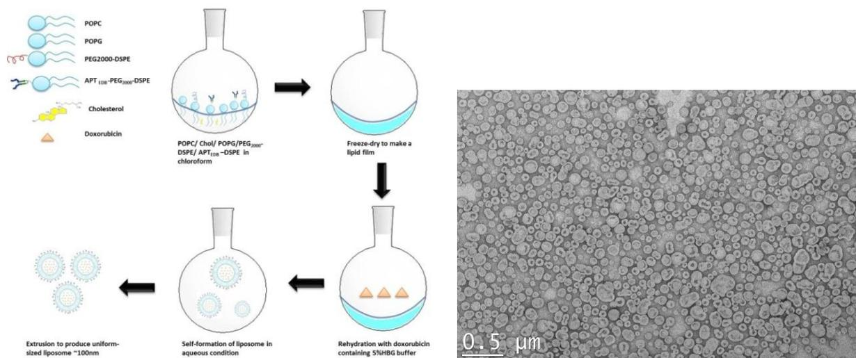
**Fig. S2** Schematic representation of liposome formation. All components were dissolved in chloroform to form a lipid film. During rehydration, Dox was included in the HBG5% buffer. Liposomes form automatically under aqueous condition. After CL-4B column purification to remove free Dox, liposomes were extruded through a 100-nm polycarbonate membrane. *Right:* TEM image of liposomes after extrusion.
