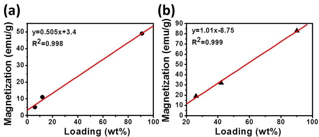
**Fig. S2.** Plot of saturation magnetization against loading wt% for MLPNs (a) 6 nm loaded samples and (b) 18 nm loaded samples.
